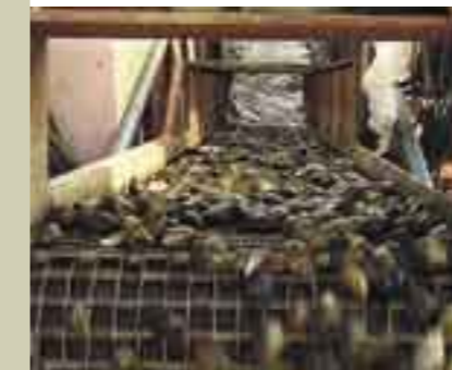
Specialised catamaran-based harvesting elevator dredge
