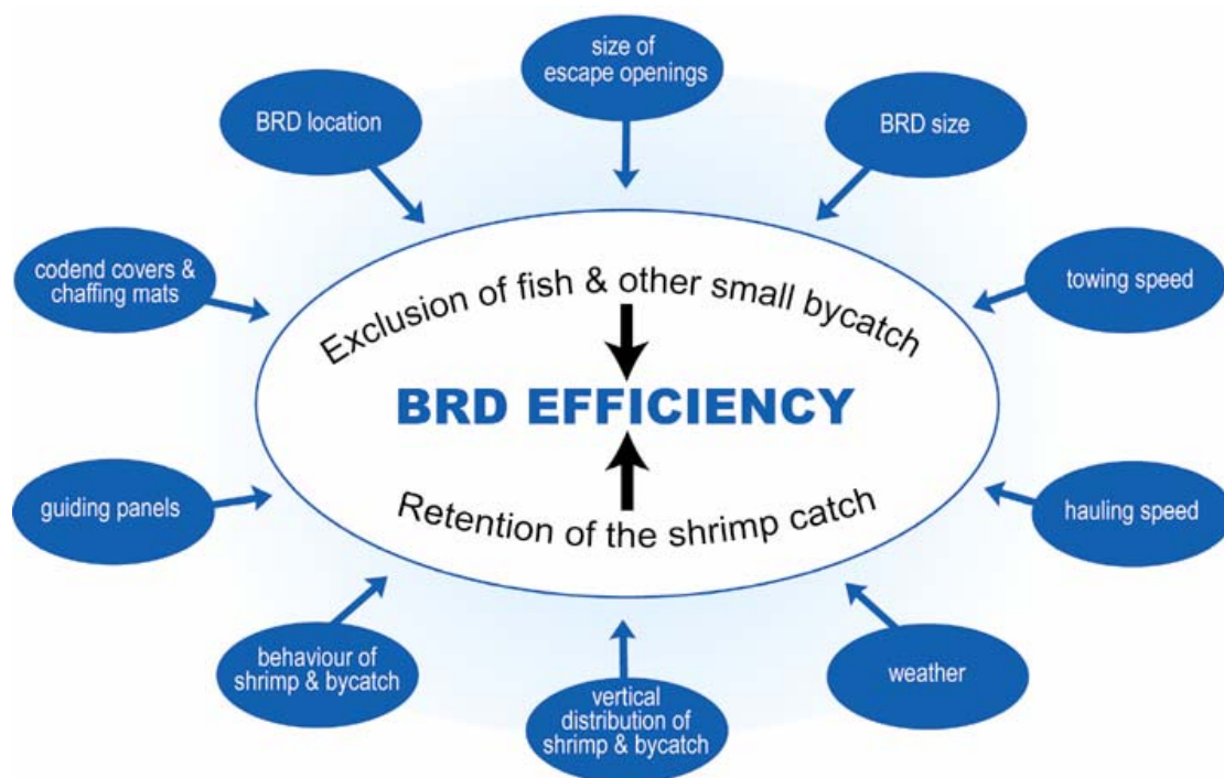
Figure 18. The various design and construction parameters that influence efficient BRD performance. Source: Eayrs, 2005.
