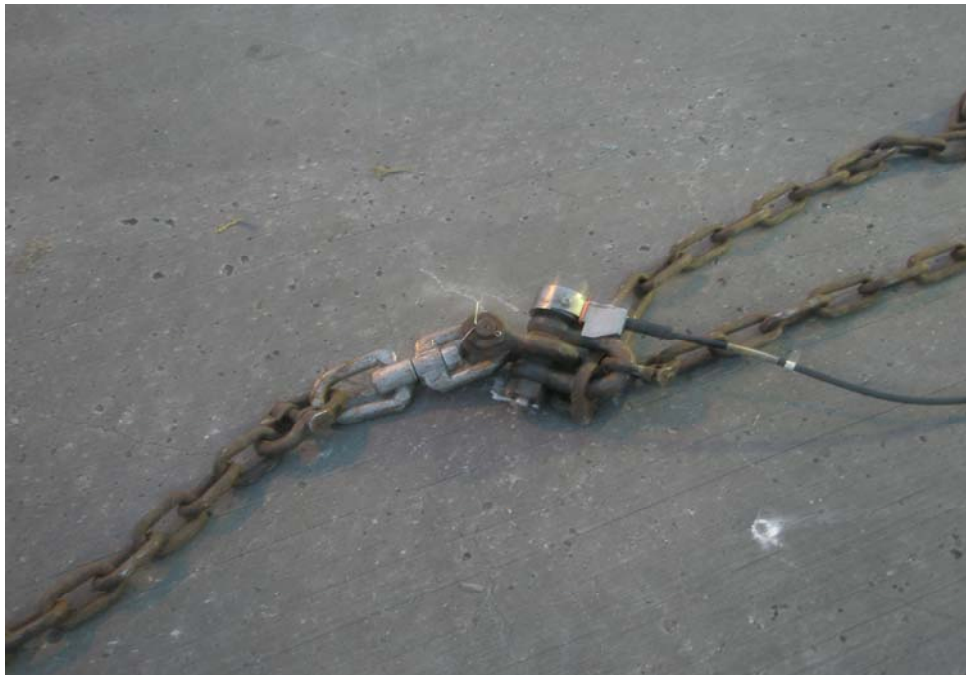
Underwater 5 ton load cells fitted to the back strops of the trawl door. The black cable leads to the Scanmar sender unit attached further up the back strop
