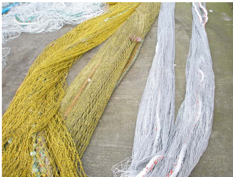
Bellies of both trawls on the pier. Left - vessels original net in 4.0 mm polyethylene netting. Right - trials net in 2.0 mm ultracross dyneema
