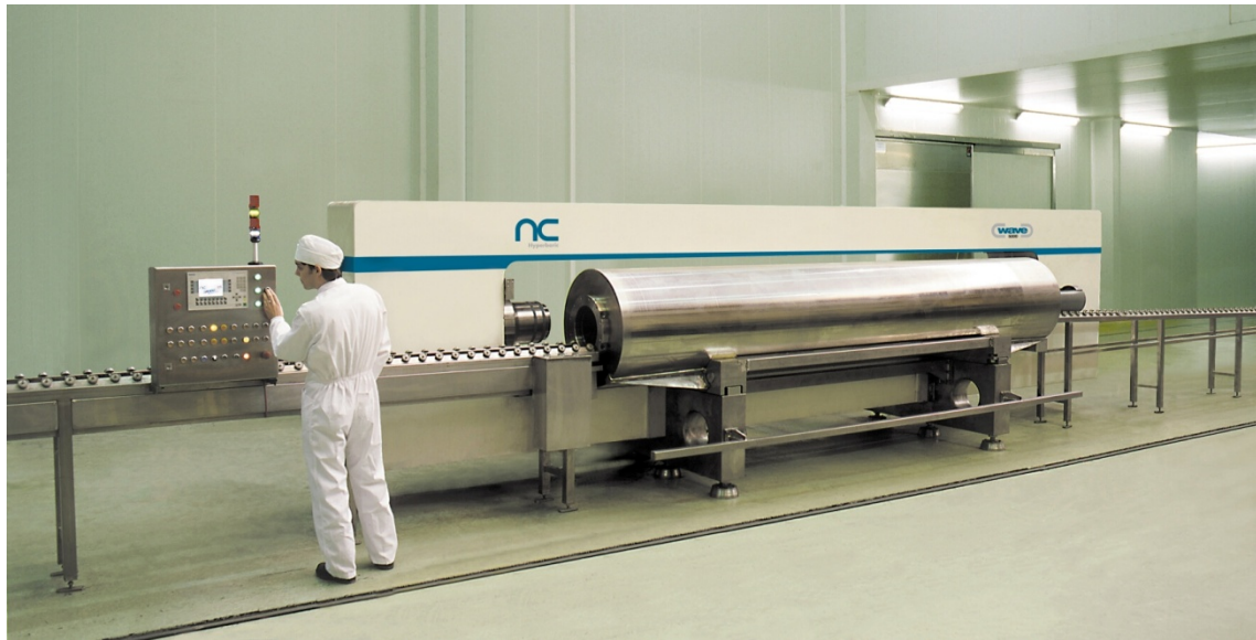
Figure 1. A horizontal batch high pressure processing vessel (picture courtesy of NC Hyperbaric, Spain)
