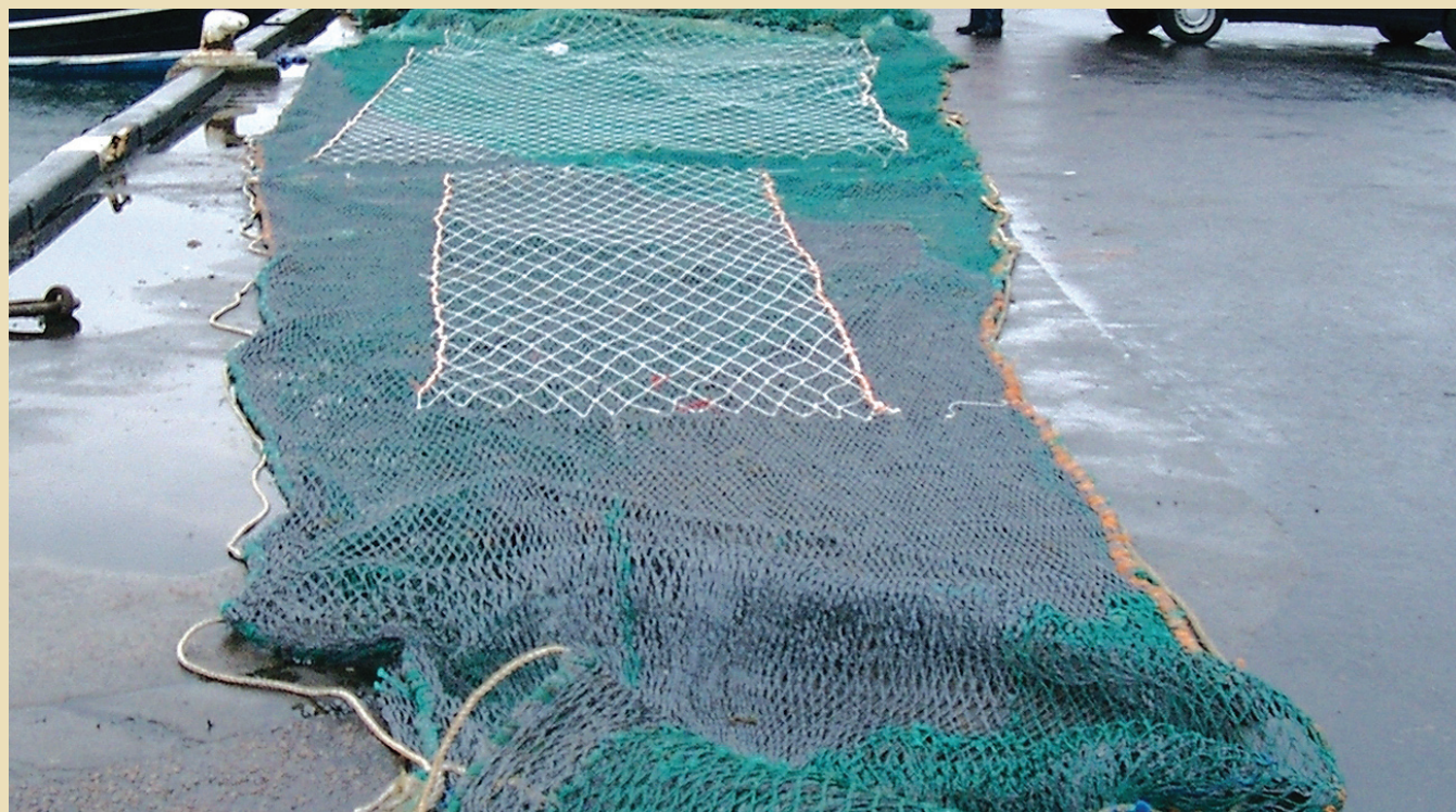
Two large mesh (300mm) diamond mesh panels fitted in a nephrops trawl
