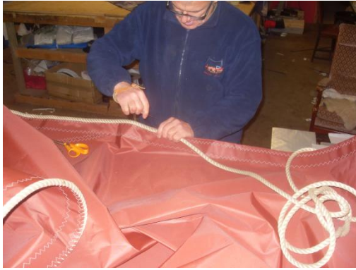
Figures 3 & 4 'Jossie' stitching in the bolt rope
