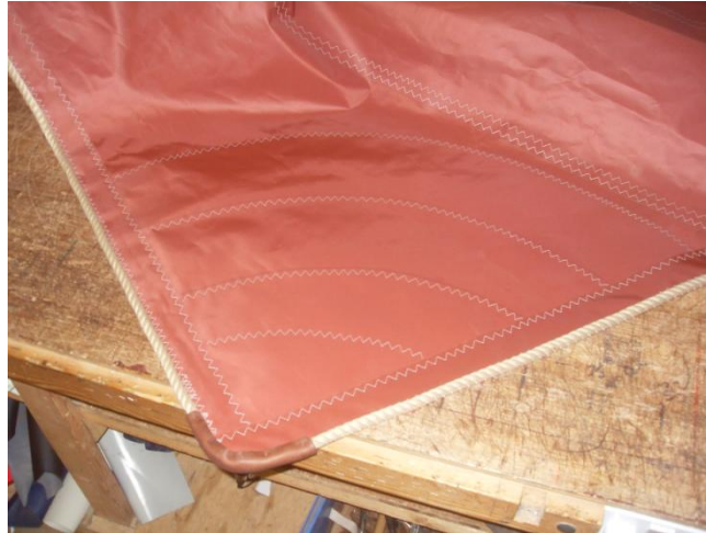
Figure 6: Reinforced sail corner
