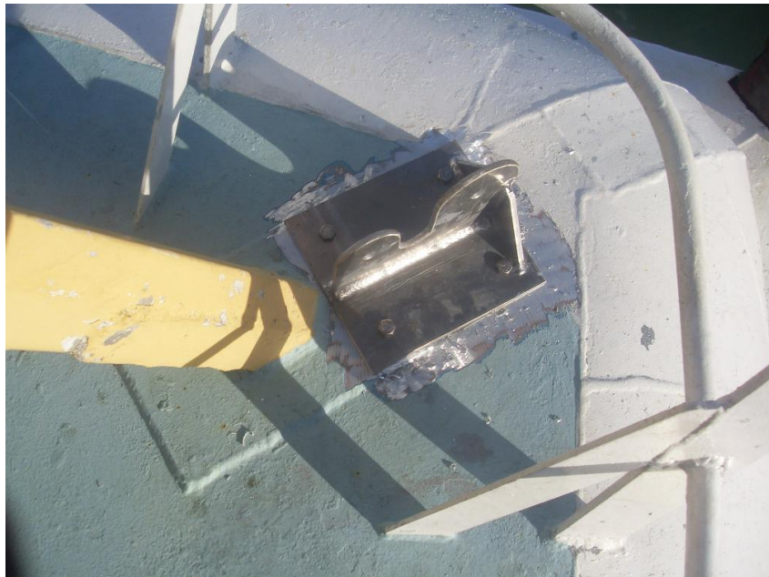
Figure 2: The mounting for the base of the forestay
