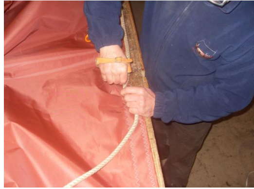
Figures 3 & 4 'Jossie' stitching in the bolt rope
