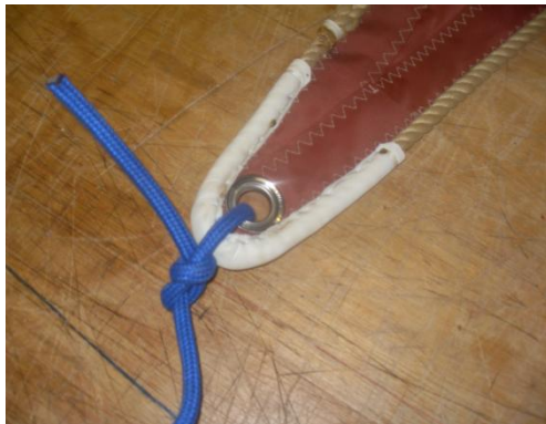
Figures 7/8: Hand stitched leather work on the sails corners
