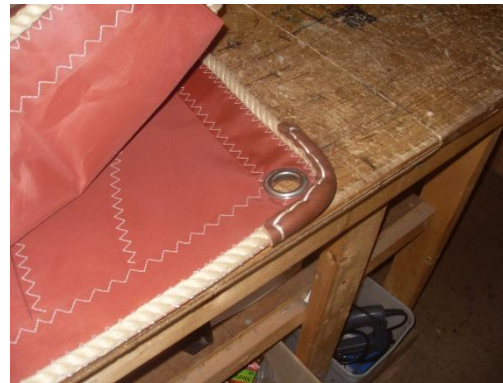
Figures 7/8: Hand stitched leather work on the sails corners
