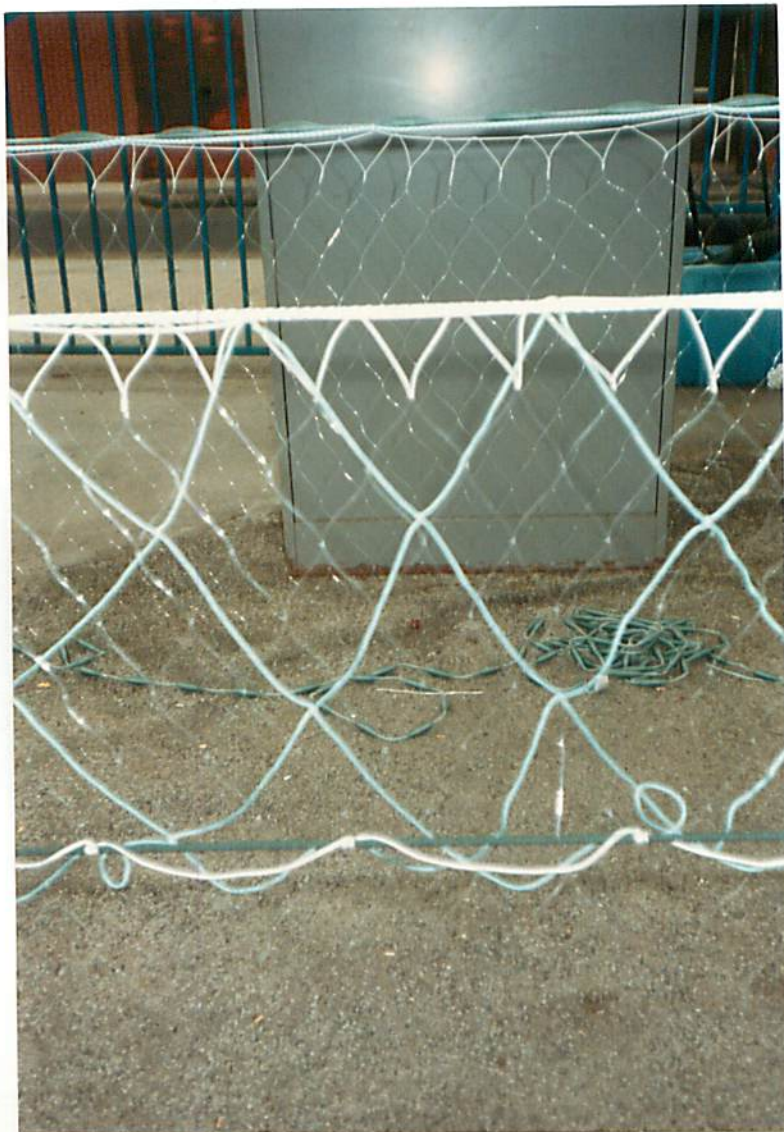
SHOWING CONSTRUCTION OF MESH BARRIER STRIP
