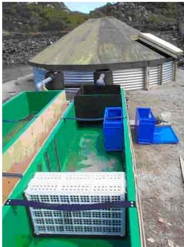
Image 5 The Tank and Treatment Trough, with initial Foam Fractionation Unit (in black)
