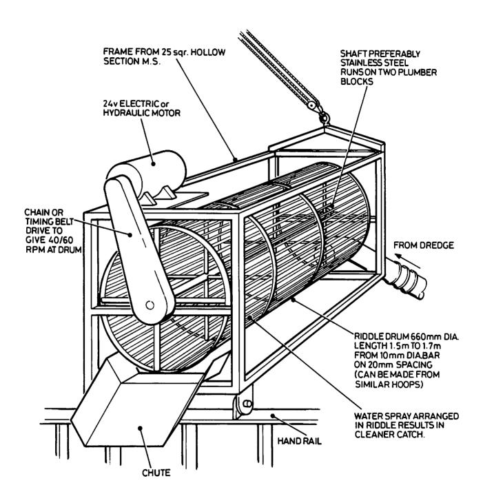
The drum is carried in a square tube frame and can be mounted over the side of the vessel, or on the deck. If the riddle is deck mounted adequate arrangements must be made for clearing the water from the deck.
