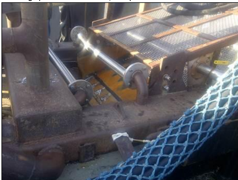
Figure 3.2. Hydraulic dredge (FCI assessment team, 2011)
