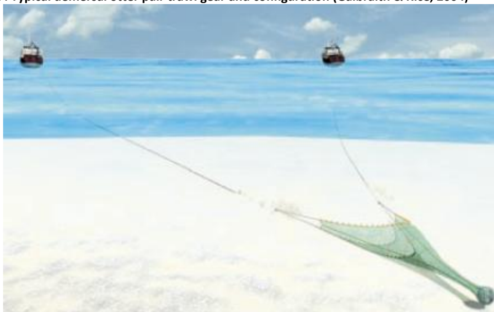
Figure 3.27: Typical demersal otter pair trawl gear and configuration (Galbraith & Rice, 2004)
