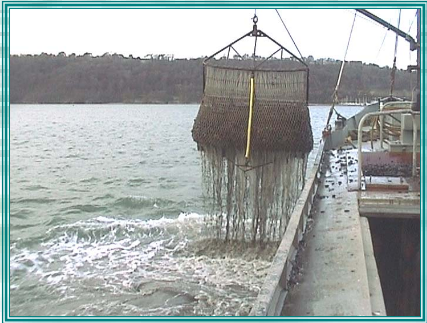
Dredges are hauled on board with a grab
