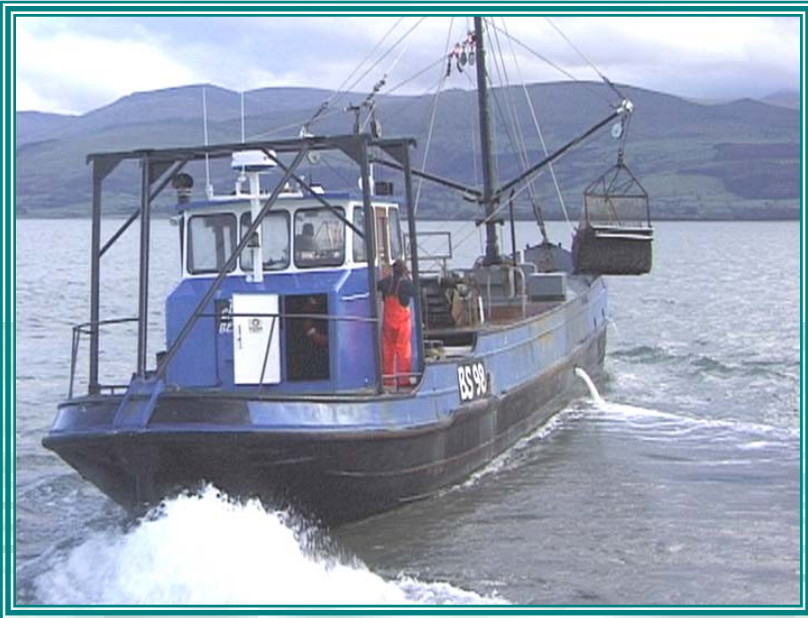
Dredges are operated from the sides of the vessel
