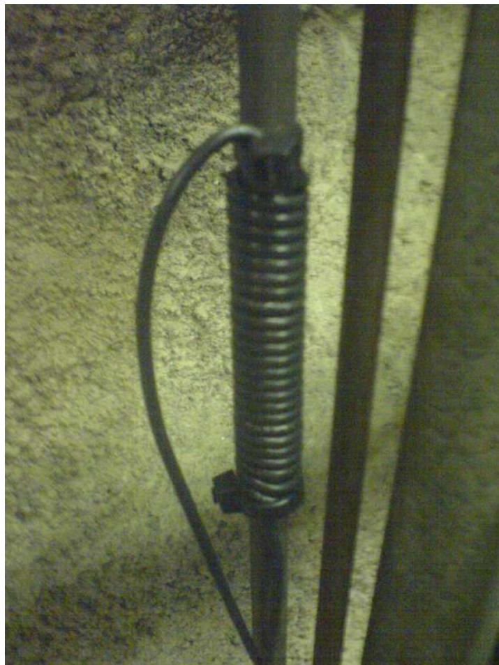
Figure 06: Detail photograph showing the electromagnetic coil wrapped around the fuel supply line to the test engine.
