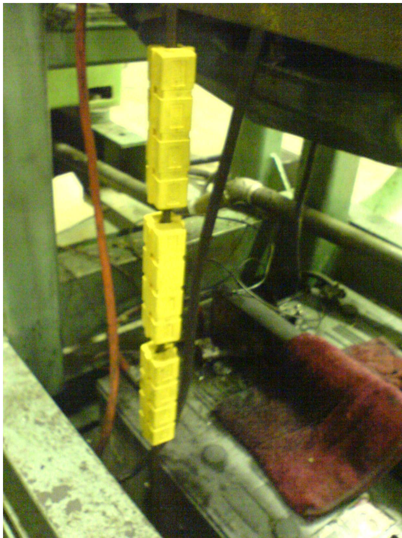
Figure 08: Three 'large' Ethos Max-power magnets installed around the fuel supply line leading to the test engine.
