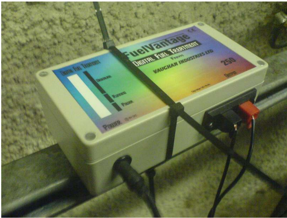
Figure 05: Detail photograph showing the FuelVantage Digital Fuel Treatment unit (Disconnected)
