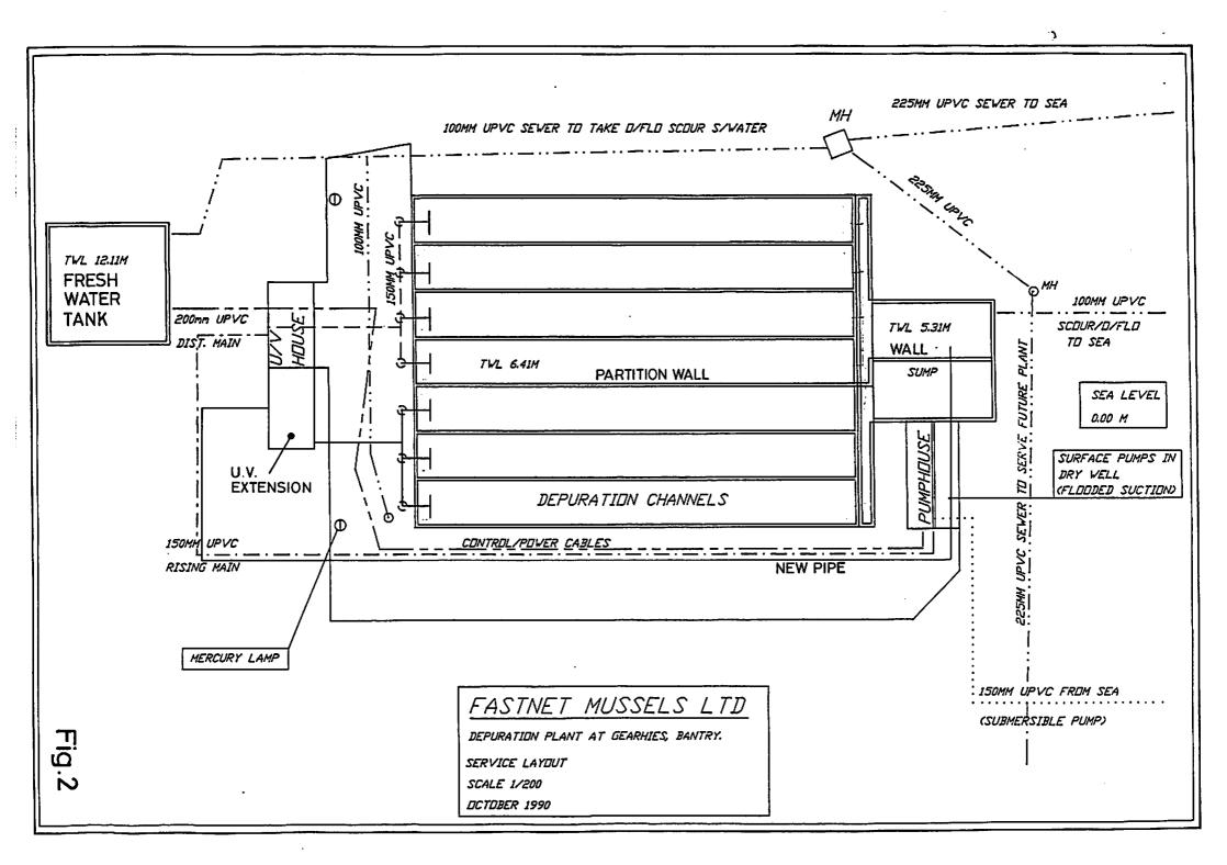
straightforward to pump direct to the channels via the u.v. sterilisers. The header tank could serve a purpose as a settling tank in case the fresh seawater is turbid (this would reduce the efficiency of the u.v. sterilisers) but otherwise we suggest it is disconnected from the purification tanks. It could instead be used as a freshwater storage tank, which the site lacks at the present time. This would have to satisfy any local health requirements.
