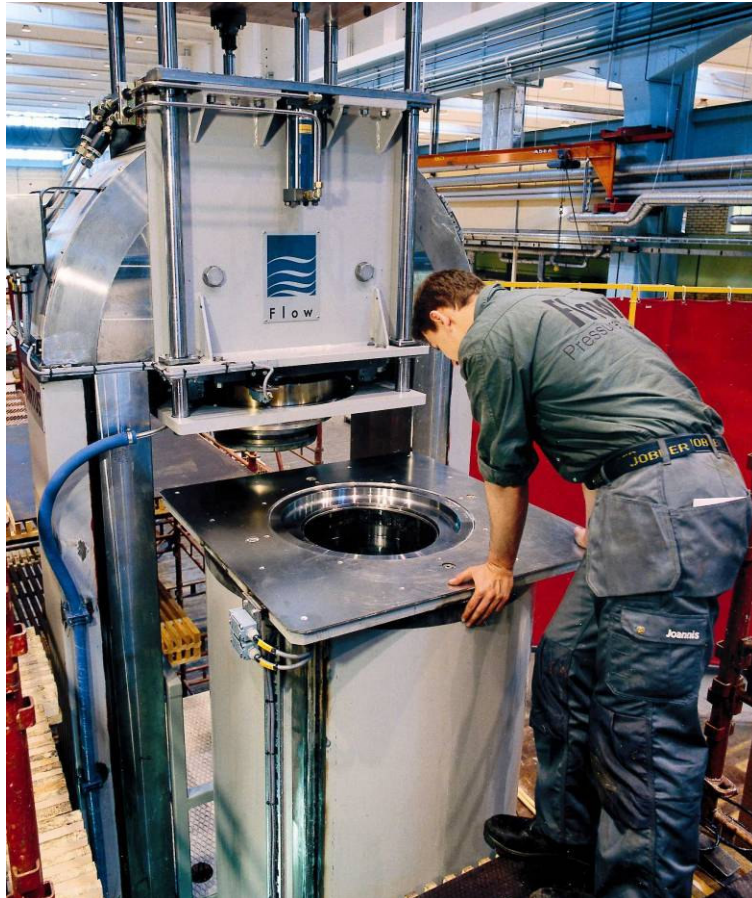
Figure 1 A vertical batch high pressure processing vessel from Avure Pressure Systems (image courtesy of Nigel Rogers, Avure Technologies)
