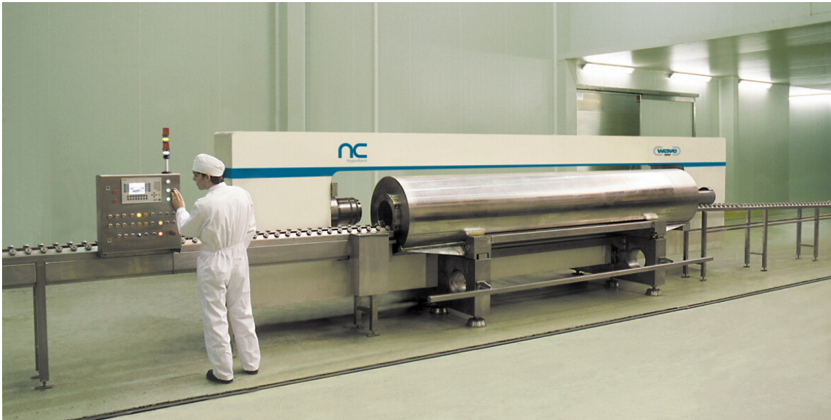
Figure 2 A horizontal batch high pressure processing vessel (covers removed) from nc Hyperbaric (image courtesy of Carole Tonello, nc Hyperbaric)
