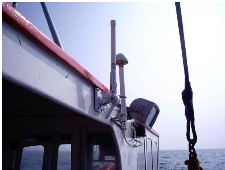
GSM & GPS aerials fitted to the MFV Palatine
