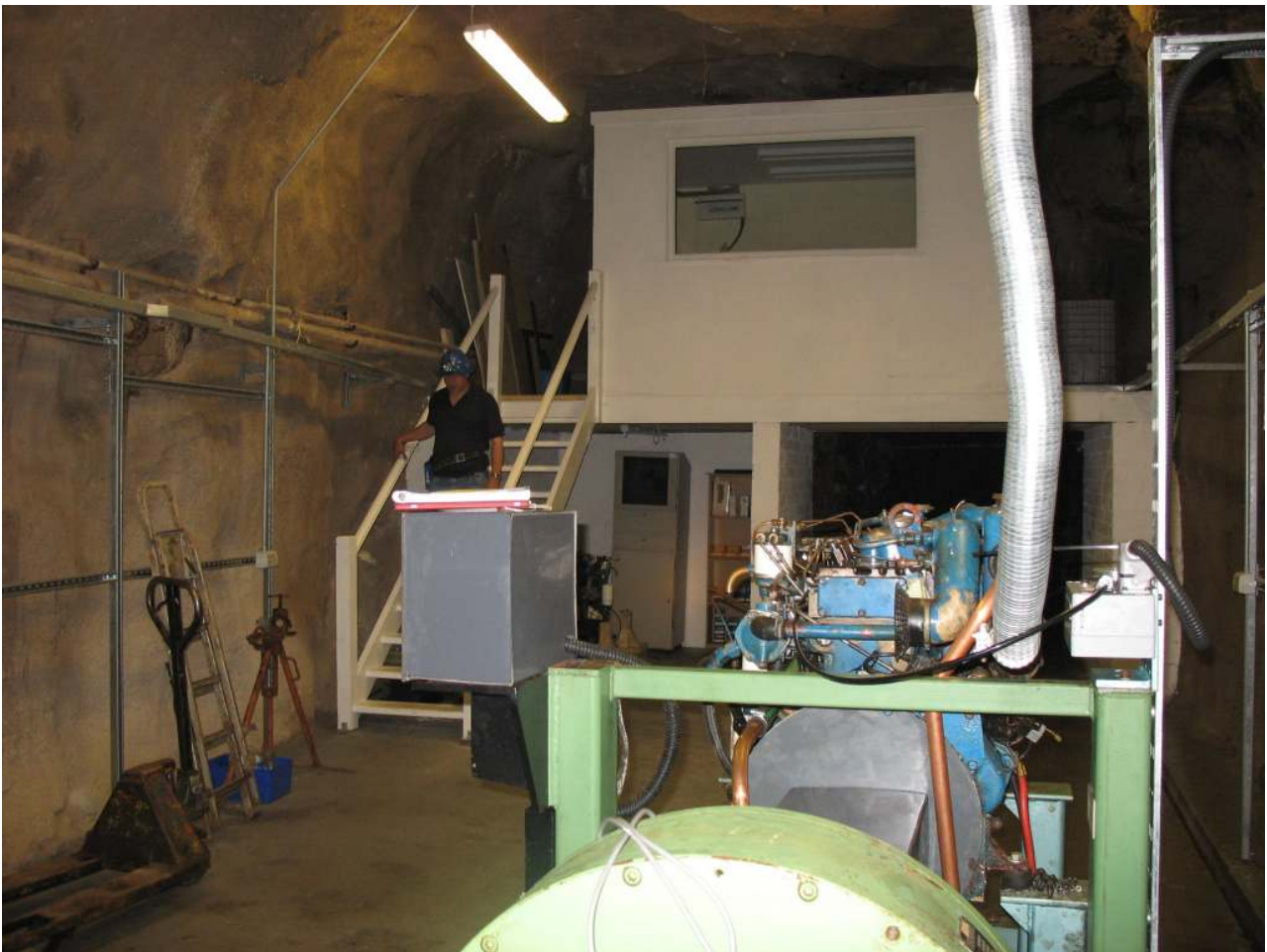
Figure 1: Photograph of the bio-fuel engine test cell facility underground at the CSM Holman's Test Mine. The top of the photograph shows the test cell control cabin. The dynamometer is in the foreground in green, the test cell engine is in blue.
