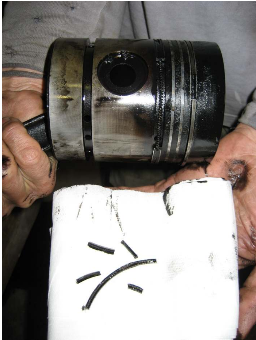
Figure 9: Broken and seized piston rings
