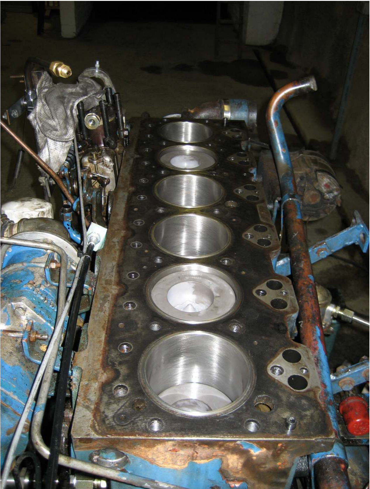
Figure 10: New cylinder liners and pistons
