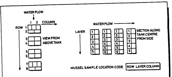
For Trial 15 a combination of two box types were used in the multi-layer tank
