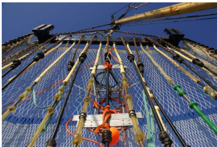
Figure 1. Measuring device placed between electrodes on TH-10.
