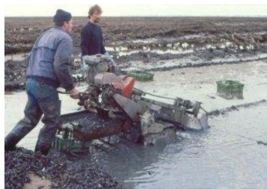
Figure 35: Mechanised methods of clam harvesting Left-hand image: Harvesting Japanese carpet shell using a tractor equipped with a blade and conveyor belt (hard bottom). Right-hand image: Harvesting Japanese carpet shell using a small tractor in small plots and soft bottom (Source: FAO)
