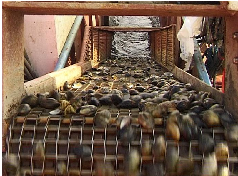
Figure 34: Elevator dredge shown harvesting clams (Source: Seafish)
