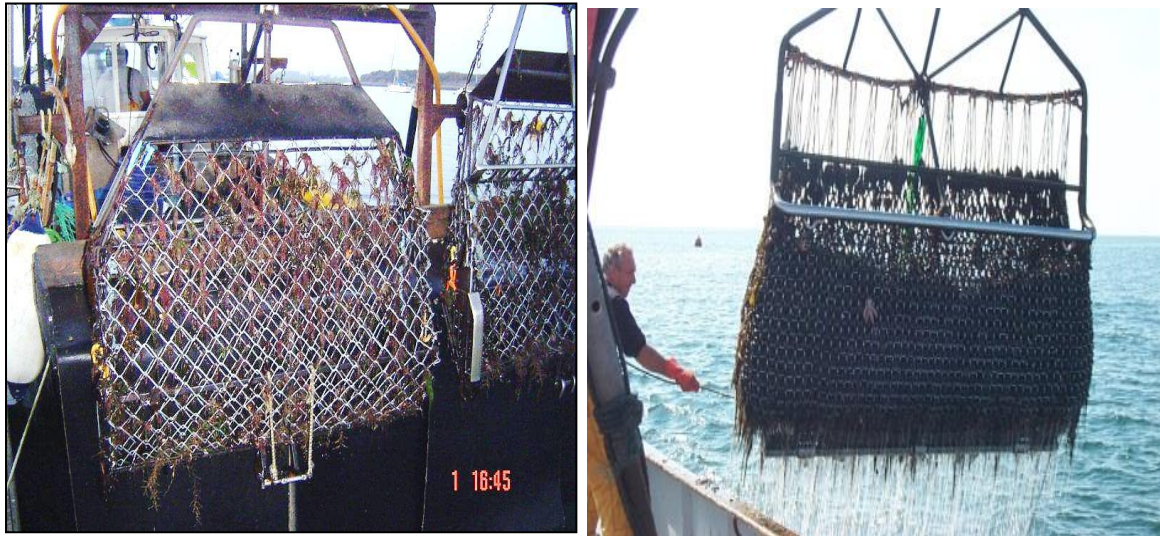
Figure 30: Heavy dredges used in shellfish harvesting. Left-hand image: Oyster dredges Right-hand image: Mussel dredge used in the Menai Straits (Sources: Sussex SFC and Deepdock Ltd.).
