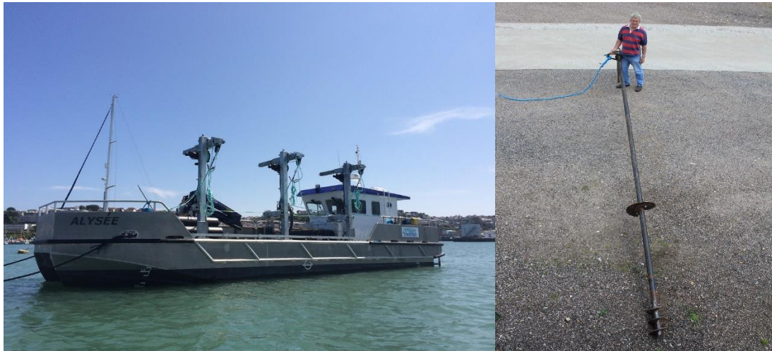
Figure 22: Screw anchor installation vessel and example of a screw anchor (Source: Offshore Shellfish Ltd. http://www.offshoreshellfish.com/ )
