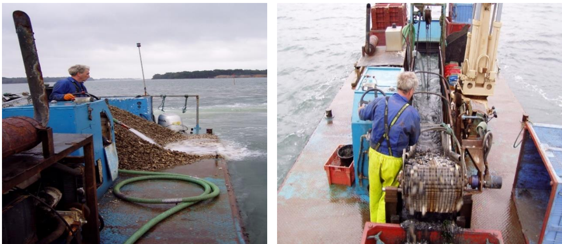
Figure 28: Eco-harvester operating on a south coast site. Left-hand image: Pacific oyster seed being spread over an on-growing site; Right-hand image: Harvesting of oysters using an elevator dredge. (Source: Aquafish Solutions Ltd.)
