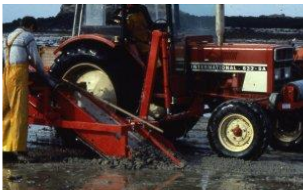
Figure 35: Mechanised methods of clam harvesting Left-hand image: Harvesting Japanese carpet shell using a tractor equipped with a blade and conveyor belt (hard bottom). Right-hand image: Harvesting Japanese carpet shell using a small tractor in small plots and soft bottom (Source: FAO)
