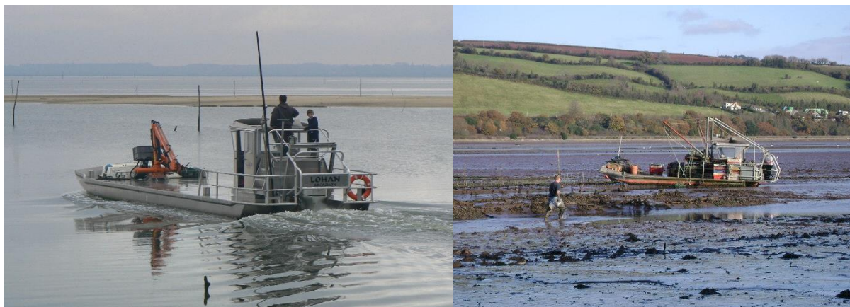
French oyster 'chaland' and similar flat bottomed vessel used in Devon
