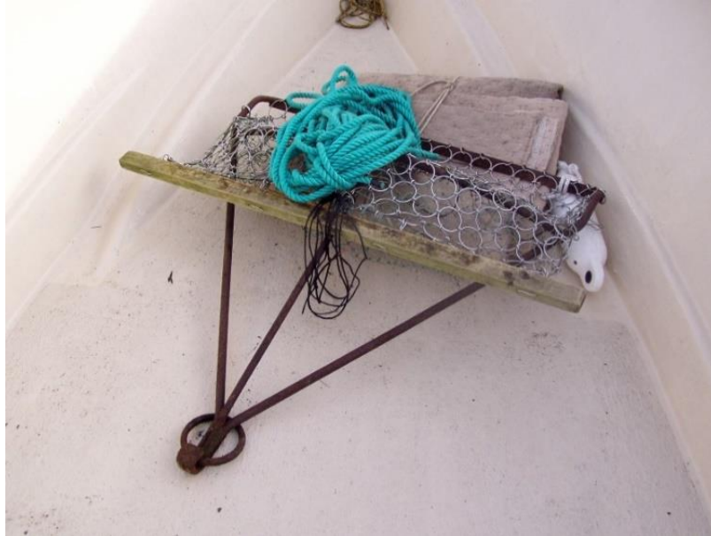
Figure 29: Traditional hand-hauled native oyster dredge from the River Fal. (Source: Salacia-Marine)
