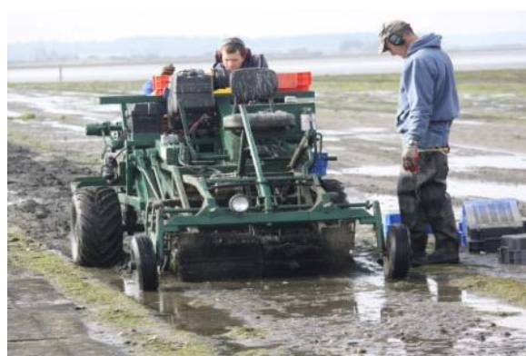
Adapted tulip harvester used for clam harvesting
