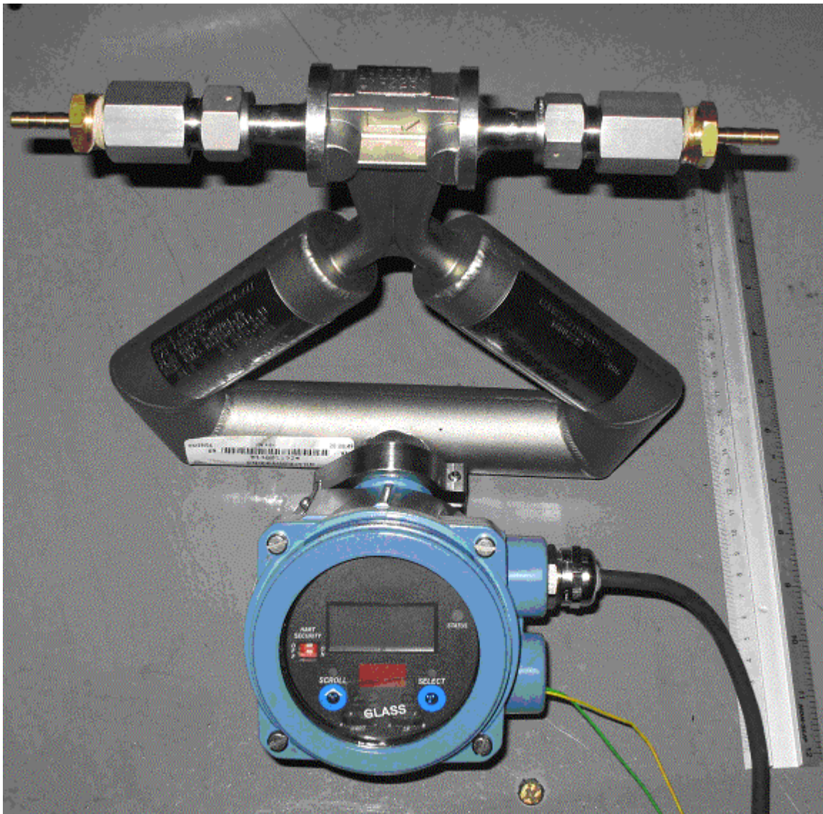
Figure 22 Emerson Micromotion Elite CMF025
