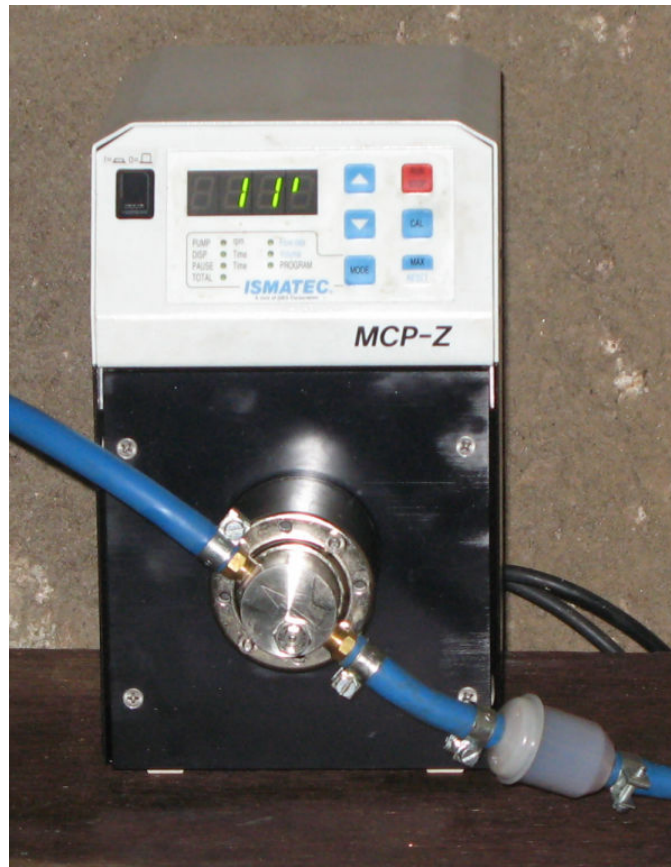
Figure 4: Constant flow rate dispensing pump, Ismatec pump drive unit & Micropump pump head
