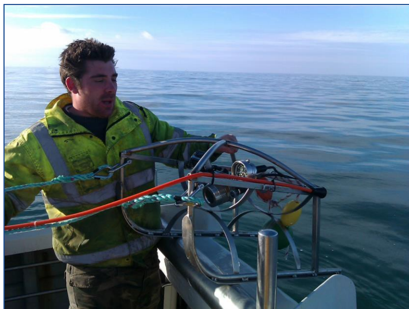
FIGURE 2. FISHERMAN NIGEL MARSH DEPLOYING THE SEAFISH CAMERA SLEDGE IN LYME BAY
