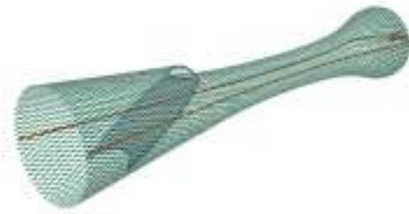
Figure 2 Schematic drawing of the inclined separator panel (Images courtesy of Fisheries Research Services (FRS), Aberdeen. Crown Copyright 2004)
