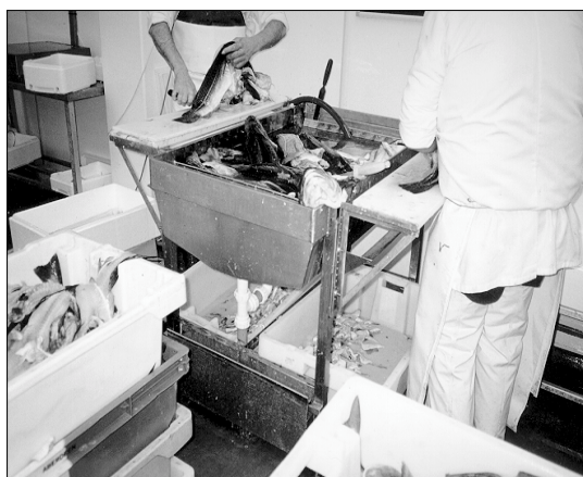
Figure 10 - Bench Design 1 Low positioned standard fishbox for trimming collection
