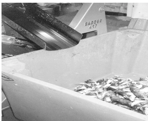
Figure 12 - Waste Collection System of the Unmodified Baader 417 heading machine
