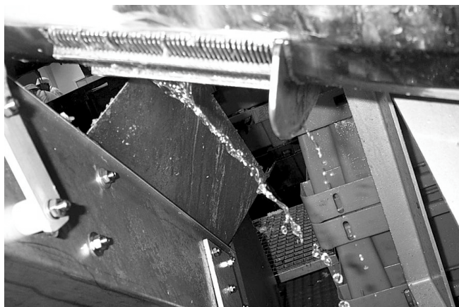
Figure 15 – Underside of the modified Baader 417 Waste Chute
