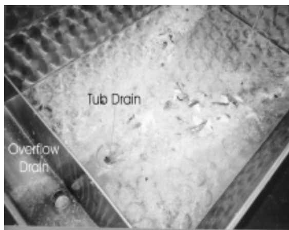
Figure 7b – Top View of the Bench Tub and Overflow
