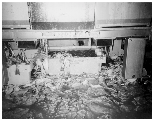
Figure 13 - Waste Collection System of the Unmodified Baader 208 filleting machine
