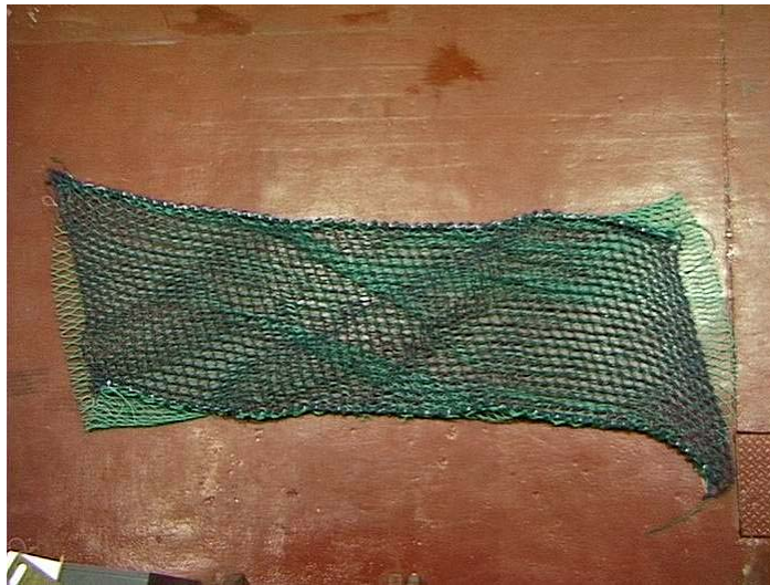
Figure 16: Double twine panel showing signs of overall panel distortion
