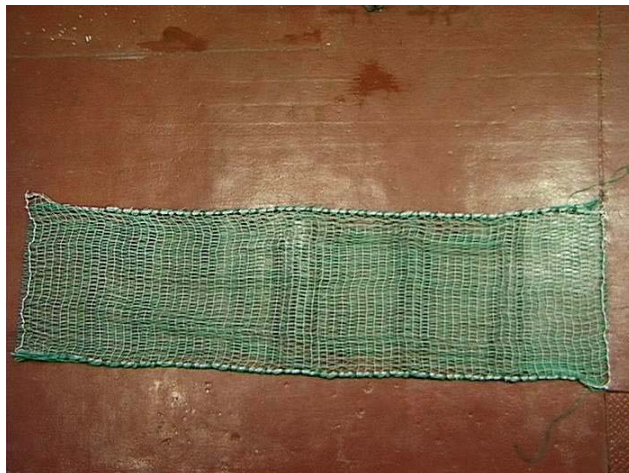
Figure 19: Dyneema panel showing overall panel shape with no distortion
