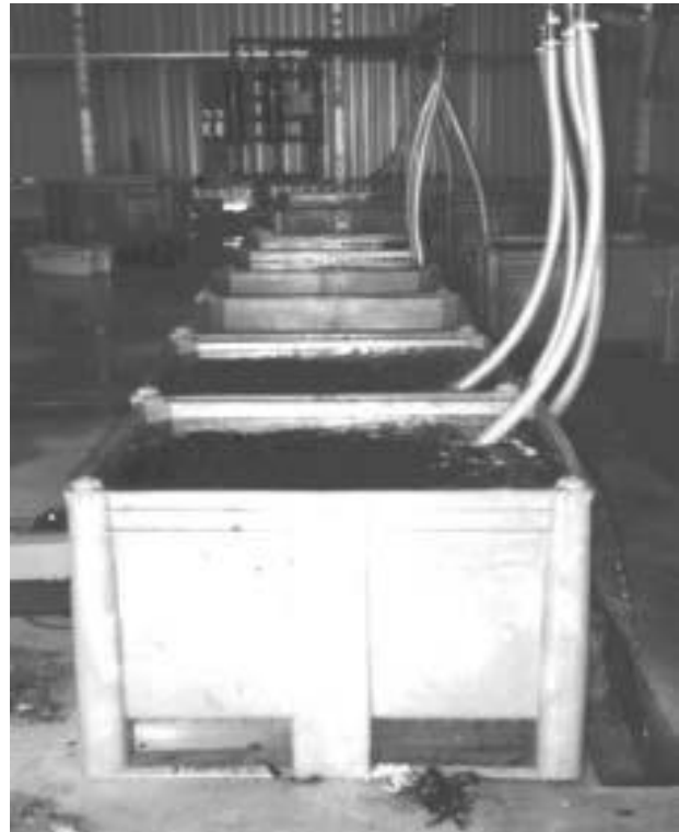
Bulk bin system for mussels
