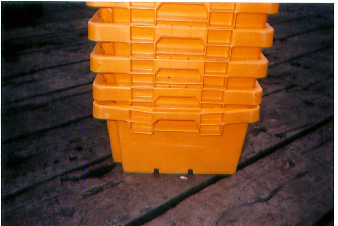
FIGURE 35 - ONE INSTANCE OF TOTAL NEST STOP FAILURE.
