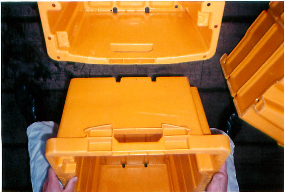
FIGURE 36 - NEST STOP FAILURE AND DAMAGE TO BOX BELOW.
