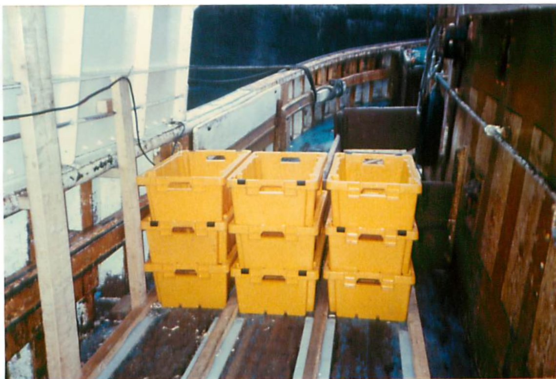
FIGURE 32 - TRACKWAY ON SUNBEAM WITH P.T.F.E. STRIPS FITTED.
