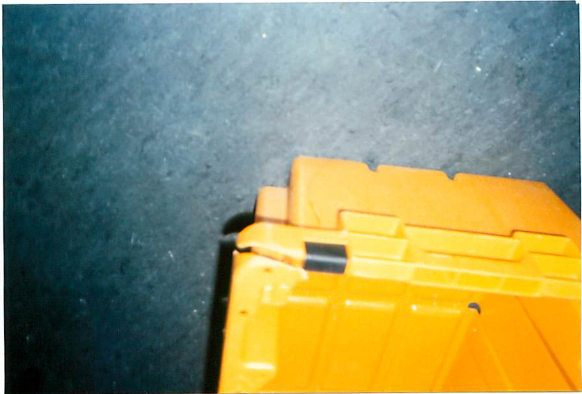
FIGURE 37 - SPLIT IN BOX CAUSED BY DISCONTINUITY OF COLOURED INDICATOR.
