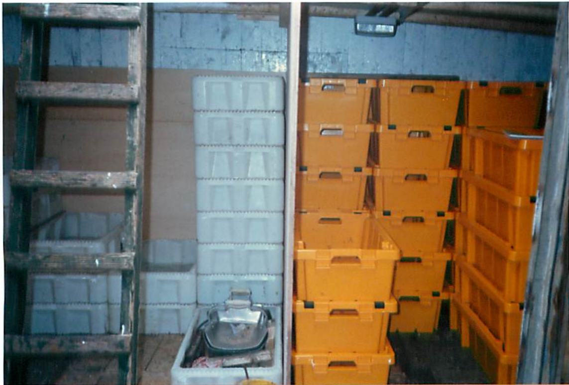
FIGURE 4 - FISHROOM PARTITIONED TO CARRY BOTH STACK ONLY AND STACK NEST BOXES.
