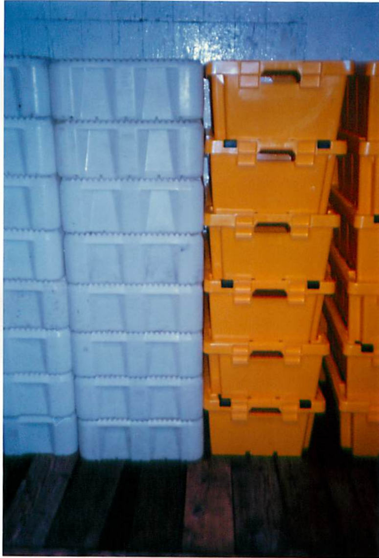
FIGURE 10 - APPARENT 25% REDUCTION IN STOWAGE SPACE BETWEEN BOX TYPES.
