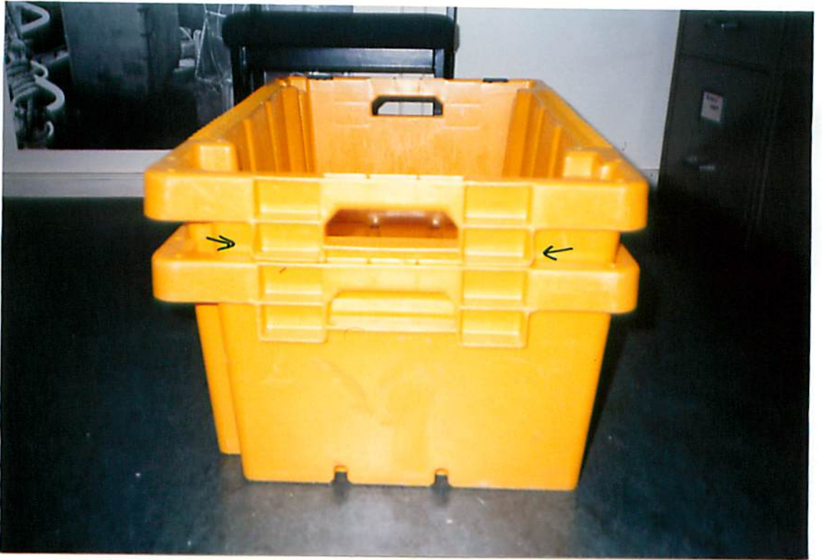
FIGURE 34 - SLIGHT BUCKLING OF NEST STOPS. (ARROWED)
