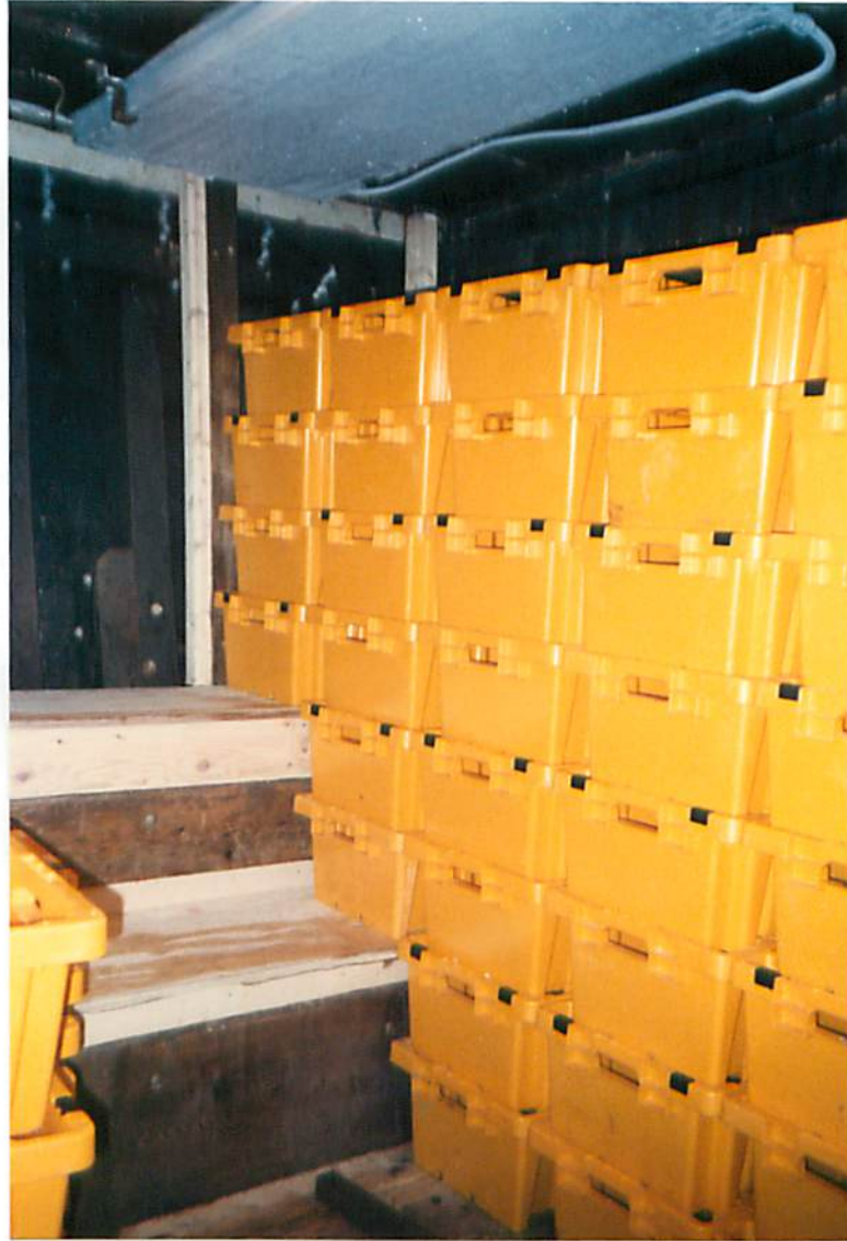
FIGURE 7 - FISHROOM STEPS ALTERED TO MAINTAIN HORIZONTAL BOX LIP CONTACT.
