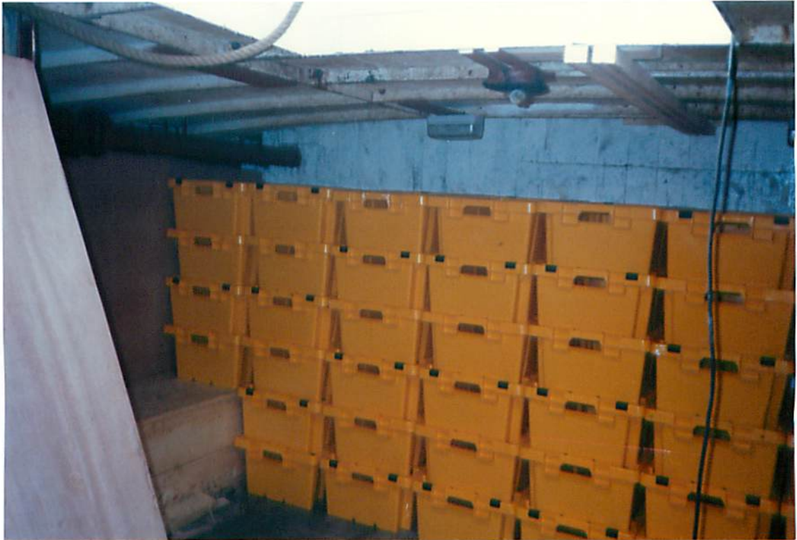
FIGURE 3 - FISHROOM MODIFIED TO CARRY STACK NEST BOXES ONLY.
