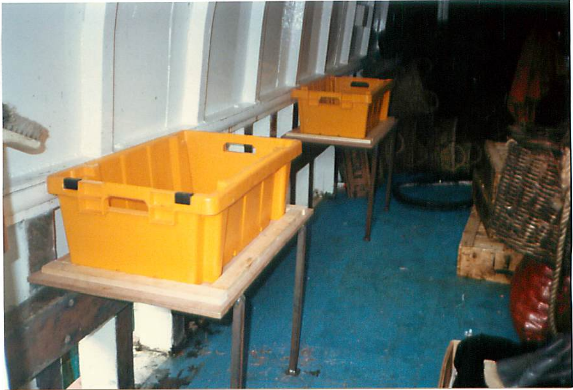
FIGURE 24 - PORTABLE BOX HOLDING BENCHES INSTALLED ON FRAGRANT CLOUD.
