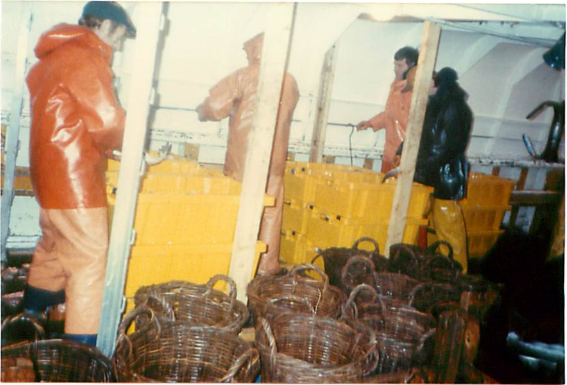
FIGURE 30 - PLASTIC BOXES SUCCESSFULLY USED ON WORKING DECK.
