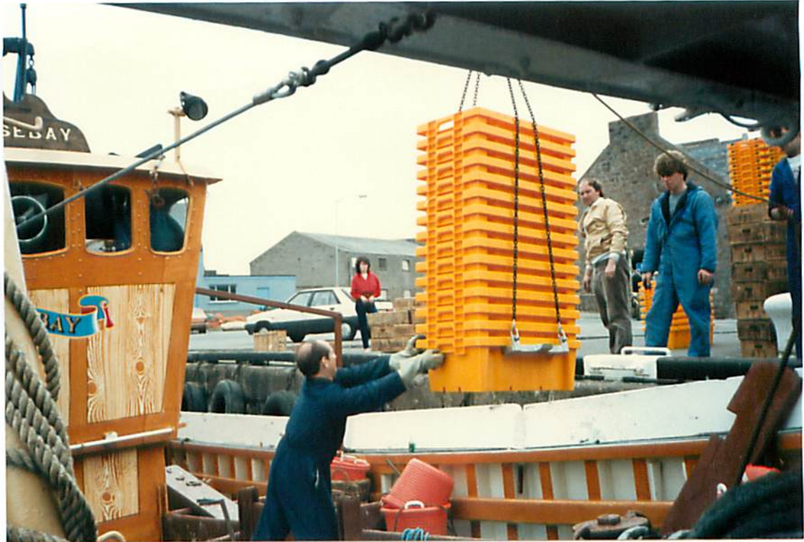
FIGURE 16 - EMPTY BOXES LOADED 15 AT A TIME ONTO ROSEBAY. NOTE FOUR POINT LIFT.
