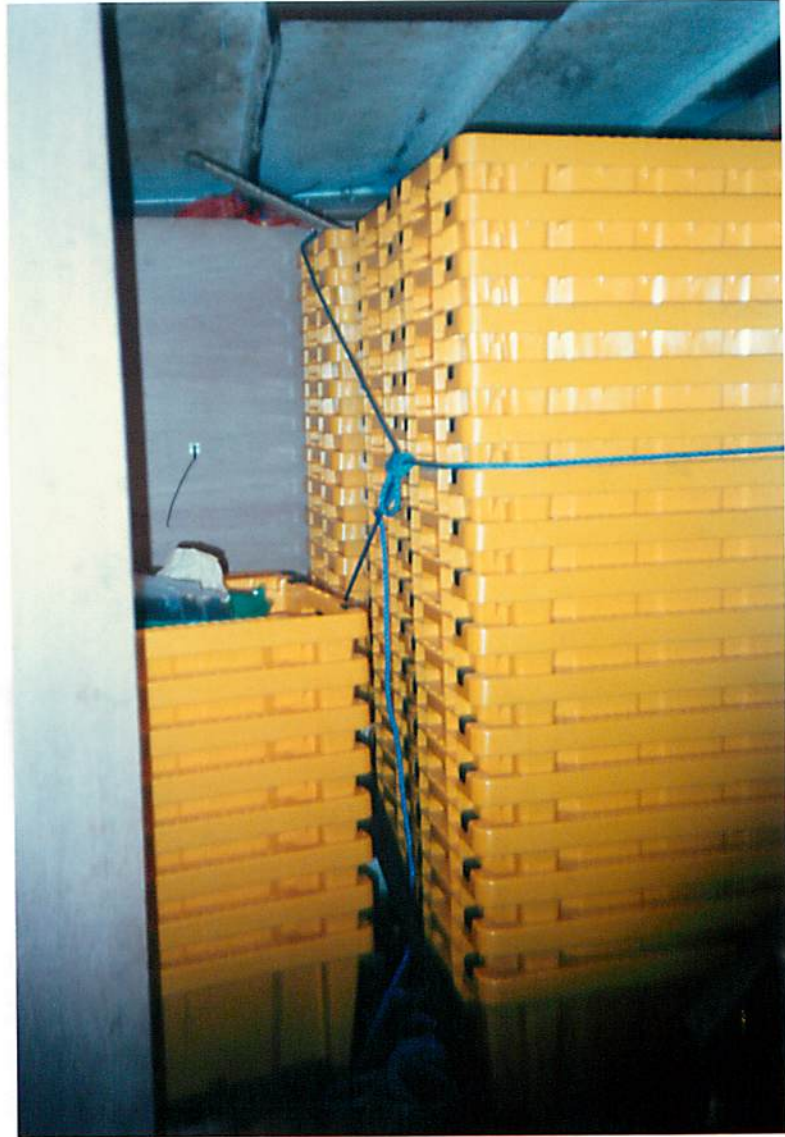
FIGURE 19 - EMPTY BOXES SECURED IN FISHROOM WITH ROPE LASHING.
