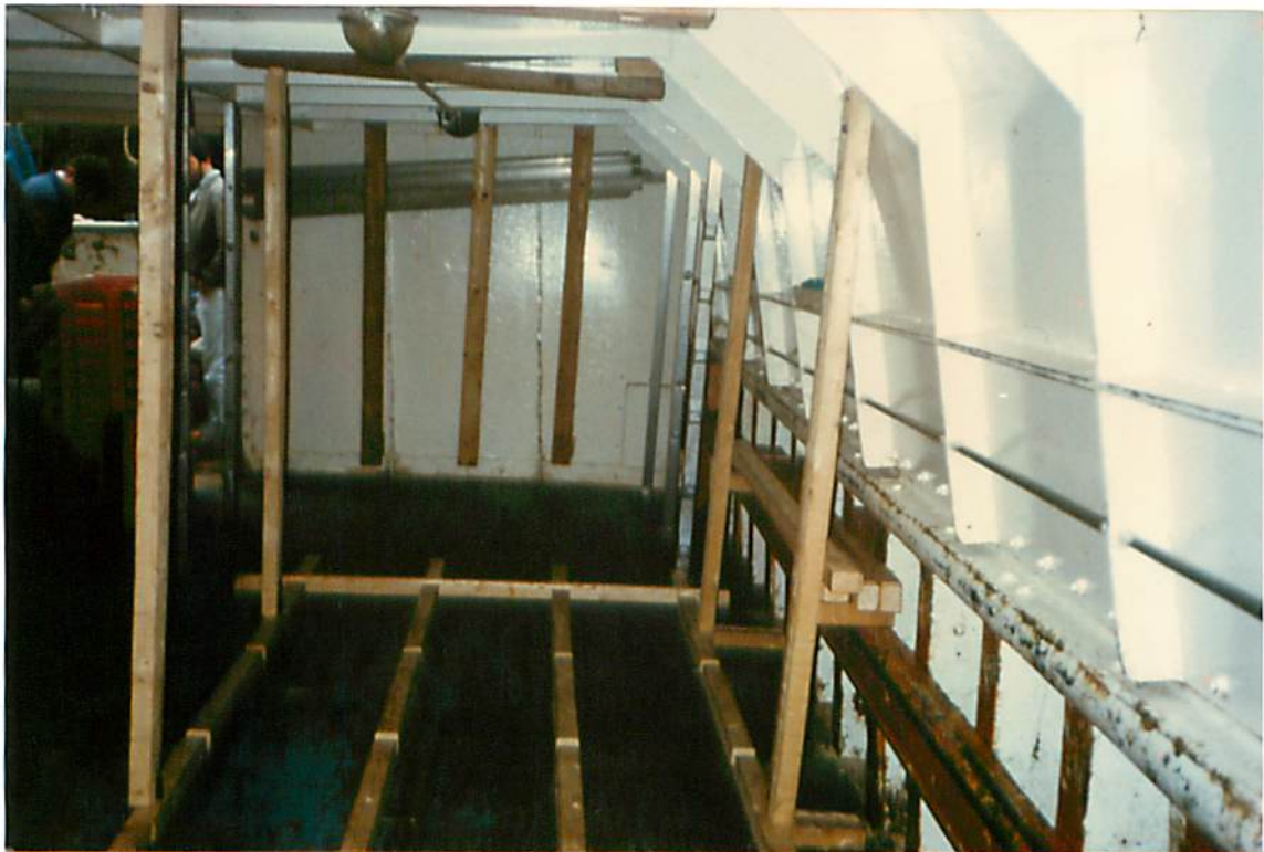
FIGURE 29 - WOODEN TRACKWAYS AND STANCHIONS FITTED TO DECK OF SUNBEAM.
