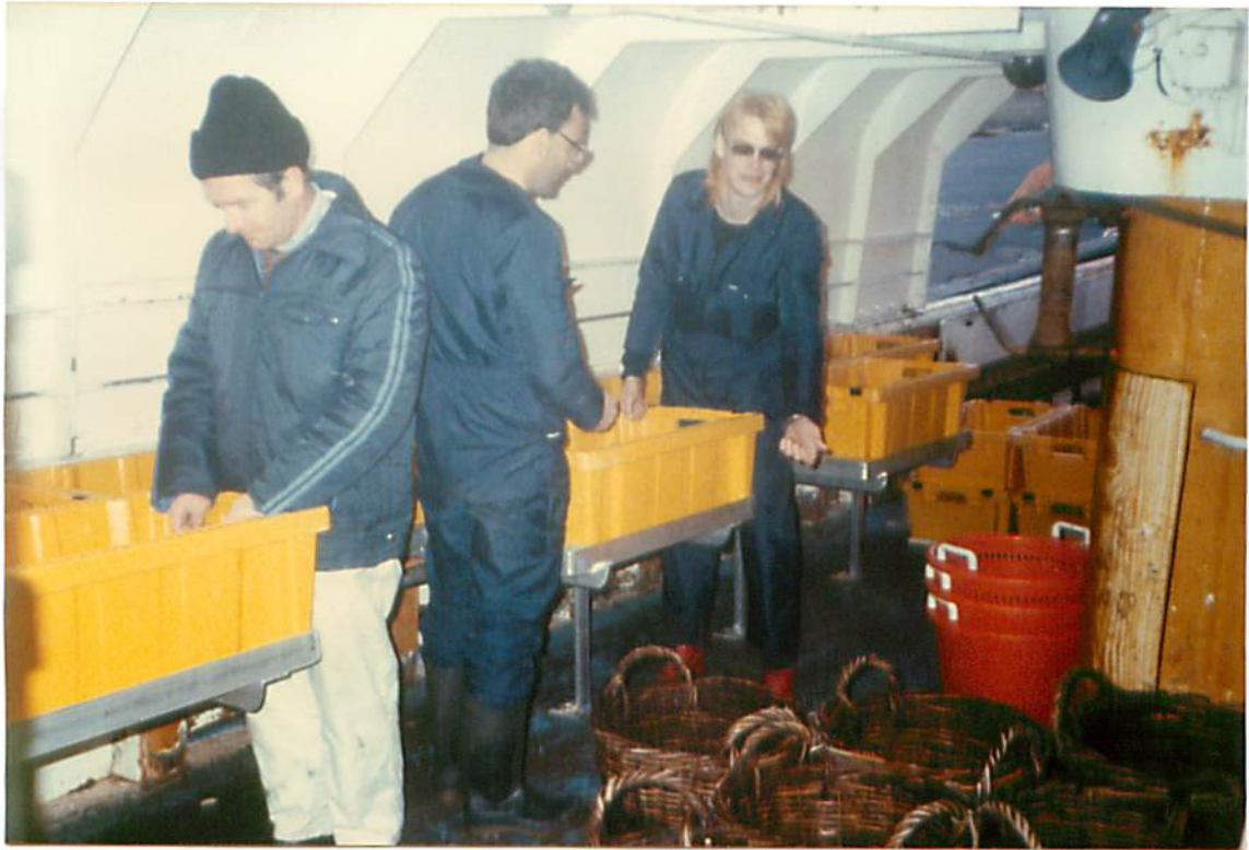
FIGURE 28 - GUTTING TRAYS ON SUNBEAM WITH BOXES IN POSITION.
