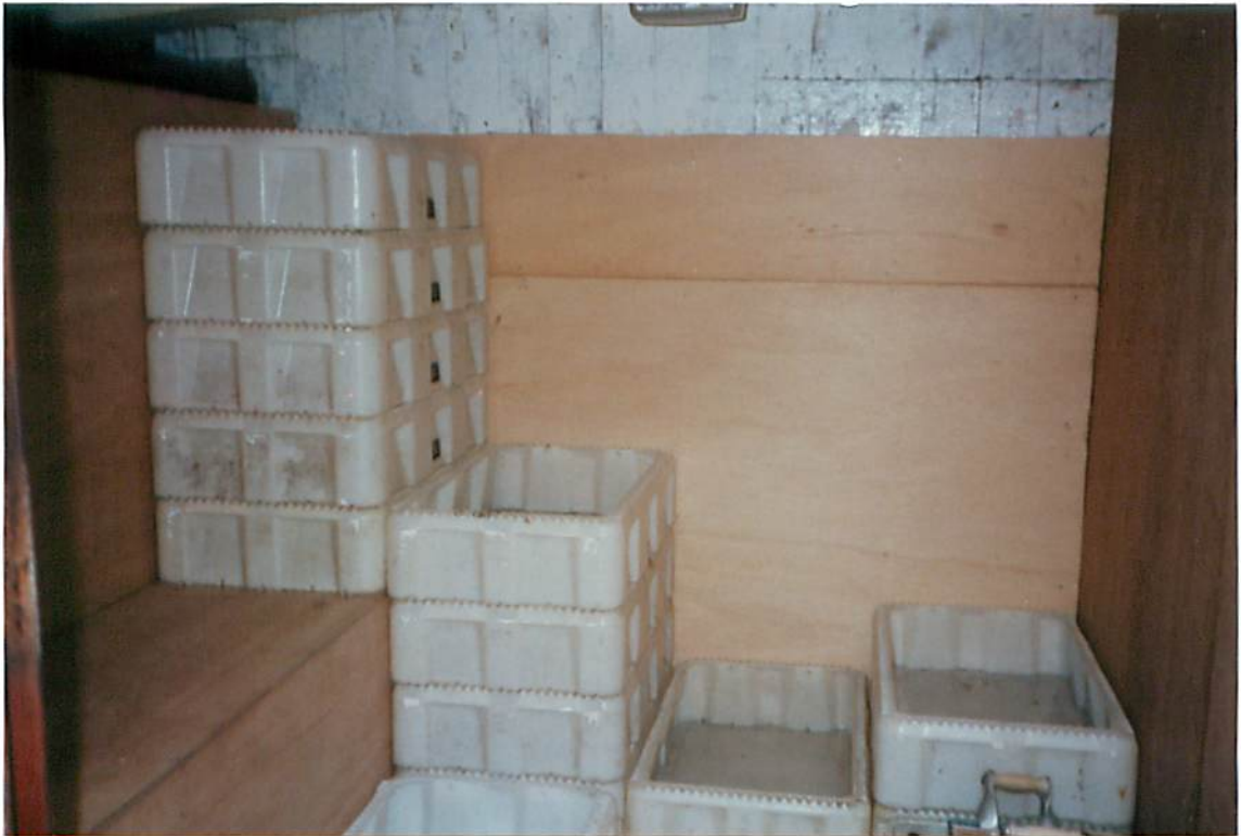
FIGURE 2 - PERS STACK ONLY BOXES IN FISHROOM LINED WITH PLYWOOD FOR TRIAL.
