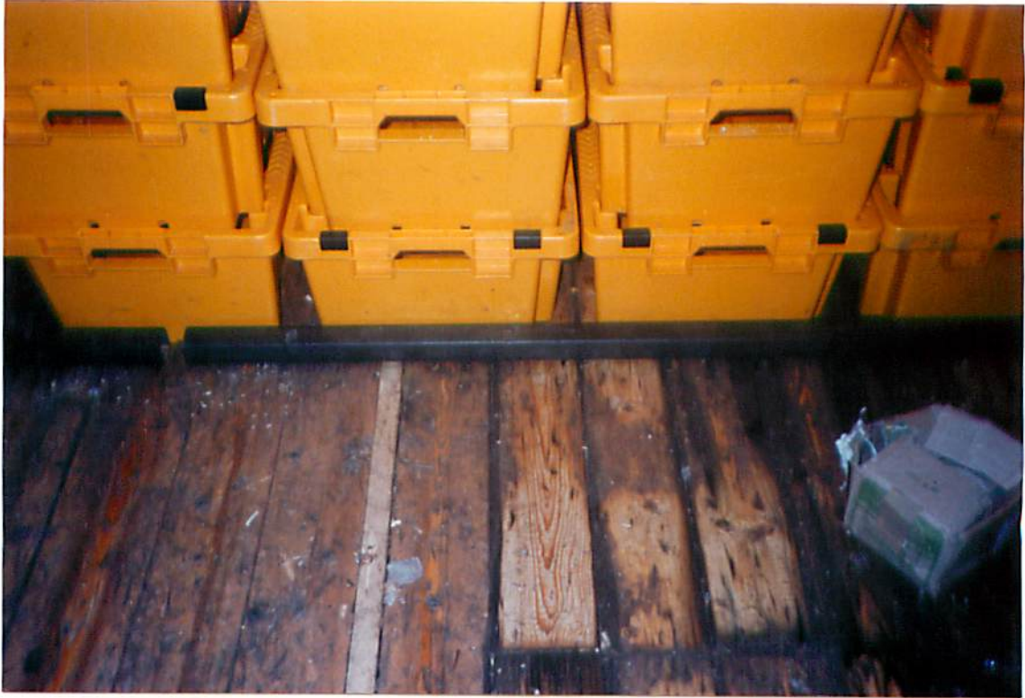
FIGURE 8 - PORTABLE STEEL STOP BARS TO PREVENT FORWARD BOX MOVEMENT.
