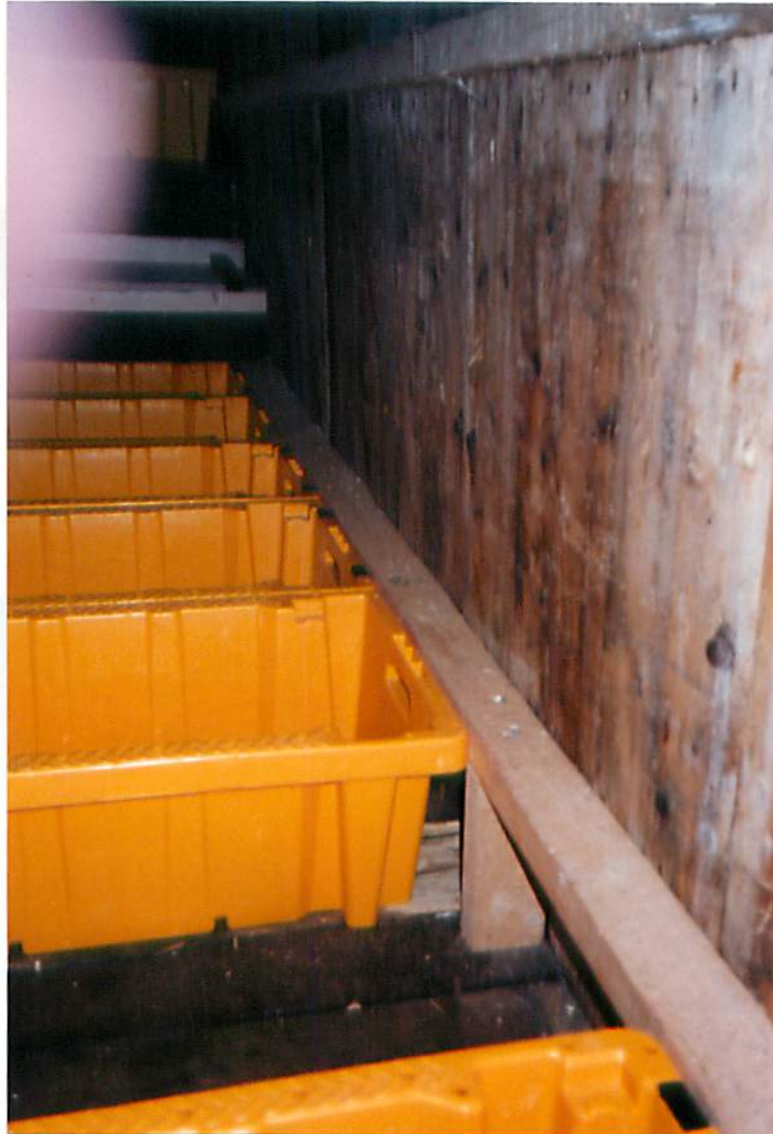
FIGURE 6 – BATTENS ATTACHED TO FISHROOM BULKHEAD TO RETAIN VERTICAL BOX STACK.
