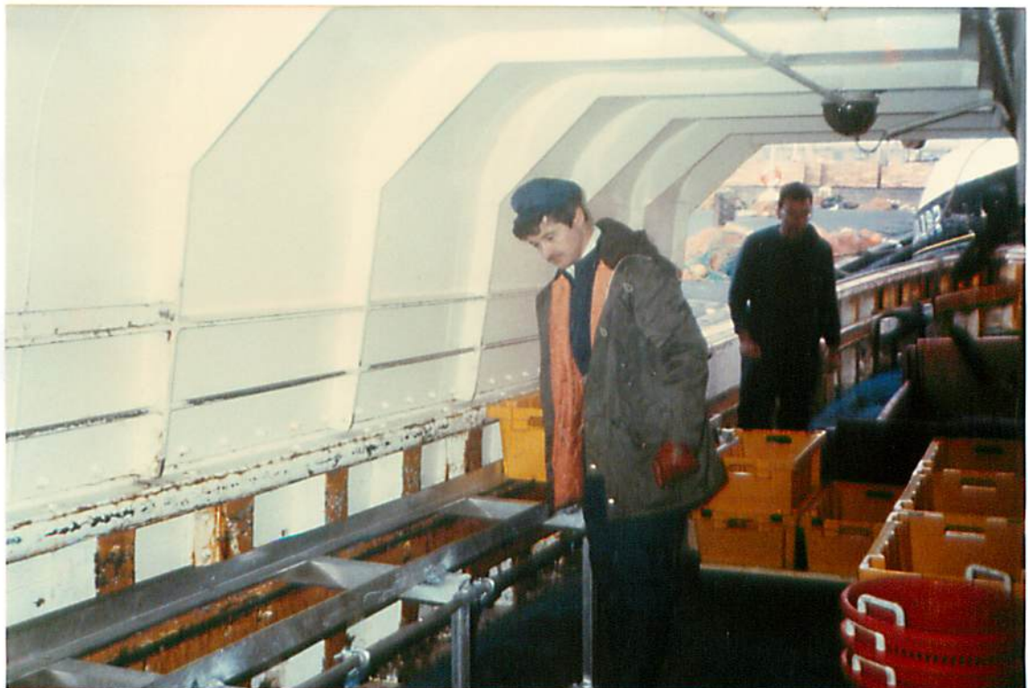
FIGURE 25 - ALUMINIUM BOX TRACK FITTED ON BOARD SUNBEAM.
