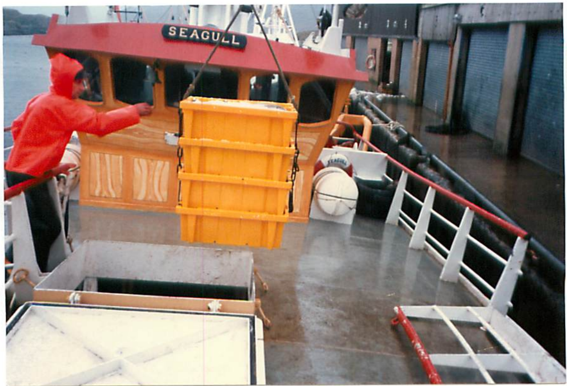
FIGURE 22 – BOXES UNLOADED FROM SEAGULL USING EXISTING UNLOADING HOOKS.
