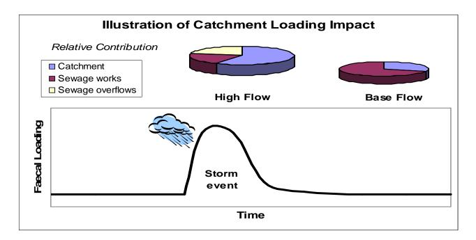
Under normal 'base' flow conditions human waste water sources may exceed catchment loads. However, under 'high' flow conditions catchment agricultural loads often dominate. Shellfish can quickly accumulate contaminants – therefore short term events can influence long term quality. With climate change and an increased potential for a greater number of more intense events this problem is only likely to get worse.
