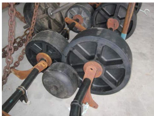
Figure 3. Size relations of bobbins used in our tests: 220 mm, 305 mm and 405 mm.
