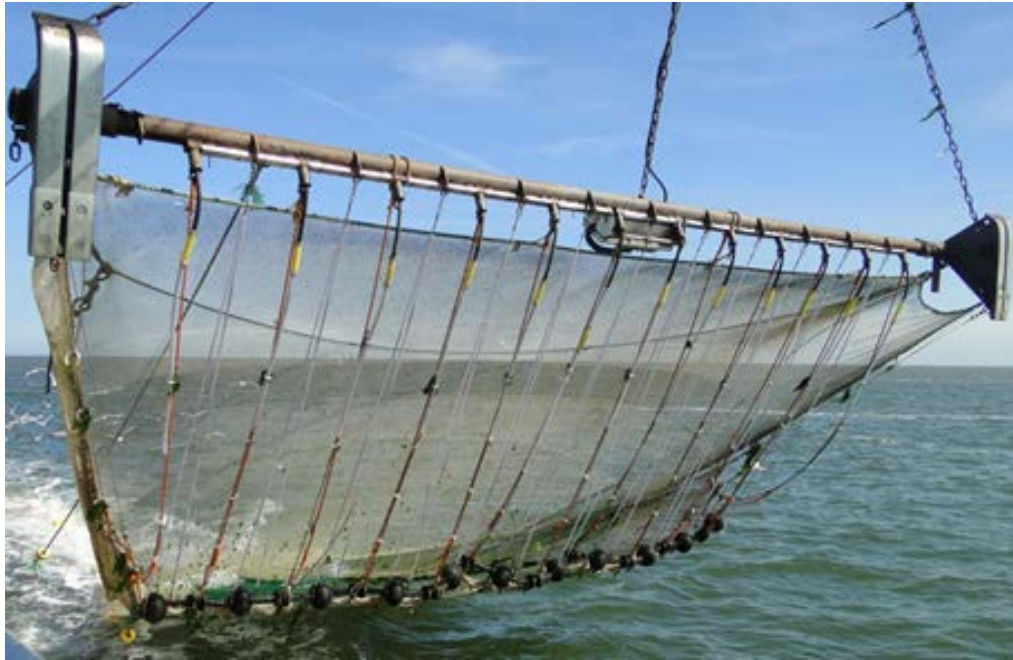
Figure 1. Shrimp pulse trawl with lightweight bobbin rope design (11 bobbins) tested on board of HA31 (Marelec pulse system).
