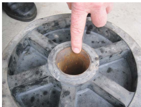
Figure 8. New challenge: deterioration of large bobbins.
