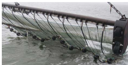
Figure 4. New challenge: deformation of the groundrope.
