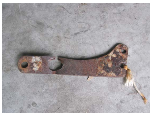
Figure 5. New challenge: weak material, breaking down of "banana"-connections.
