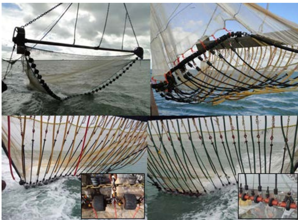
Figure 2. Different groundrope designs tested on board of TH10 with the DELMECO COMBIPULSE system.
