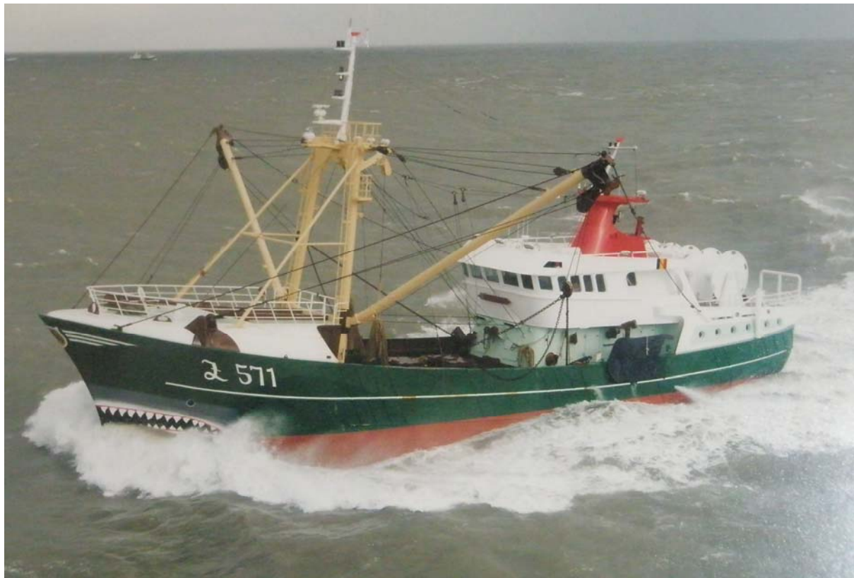
Belgian beam Trawler converted to use twin rig as well as beam trawls.
