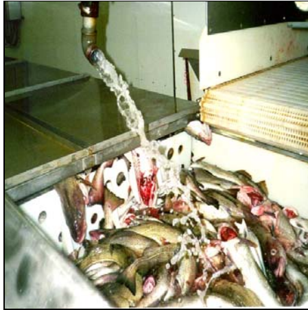
Figure 22 - Binary ice being pumped onto cod on the conveyor at the top of the cooling tanks
