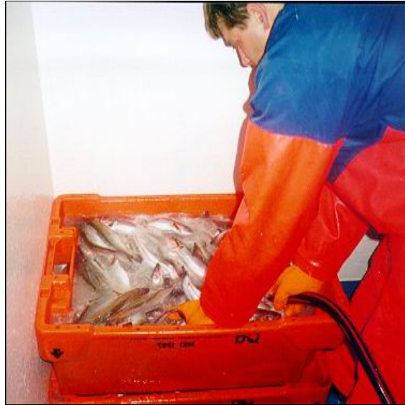
Figure 20 - Dispersing binary ice throughout a box of fish in the fish room of the vessel
