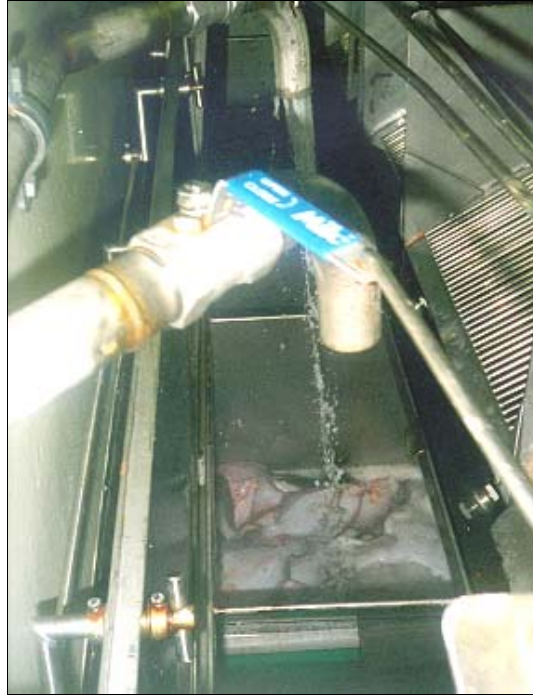
Figure 19 Binary ice flowing onto top of fish in a pre-cooling tank on the vessel
