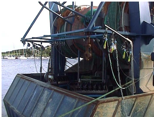
Fig 12 Stern area of 'Les Marquises' SO899, an Irish based trawler fitted for albacore trolling
