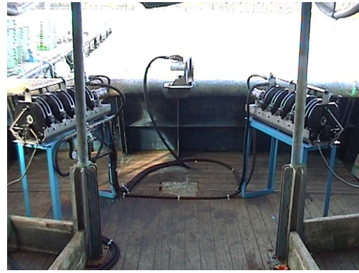
Fig 11 Deck arrangement for five reel system
