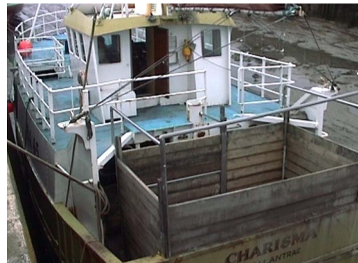
Fig 19 The net pounds at the stern of the 'Charisma' would need to be removed to accommodate the trolling reels. Poles would mount directly on the deck shelter
