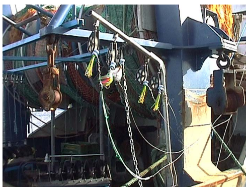
Fig 14 The fairleads that guide the nylon lines out over the side of the boat to the trolling poles
