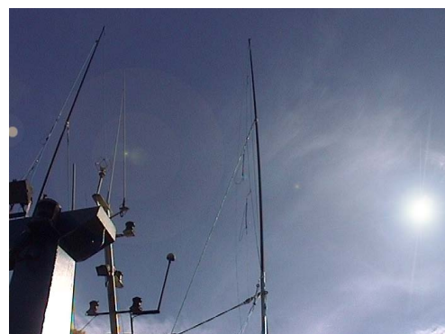
Fig 15 The trolling poles on 'Les Marquises' in steaming position. These are aluminium with carbon fibre tips
