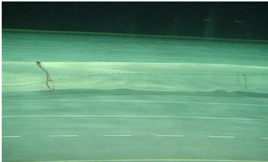
Figure 11: Showing ‘rippling’ effect created by differences in mesh opening between top and bottom panels
