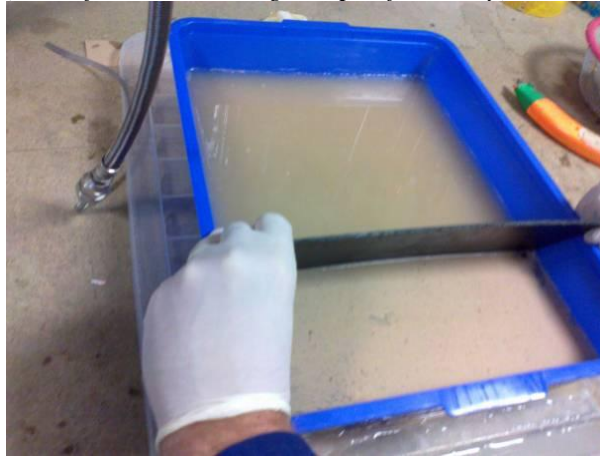
Plate 3.11 Dissolved Air Floatation of Crab (Note: flesh scum being scraped from tray)
