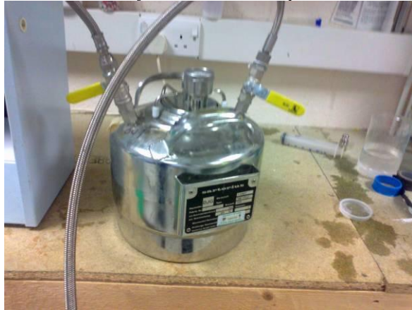
Plate 3.9 Pressure Vessel for 'White water' production
