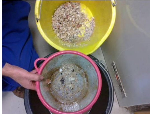
Plate 3.12 DAF Cleaned Shell and Separated Flesh (Note: Numerous crab eyes in flesh fraction)
