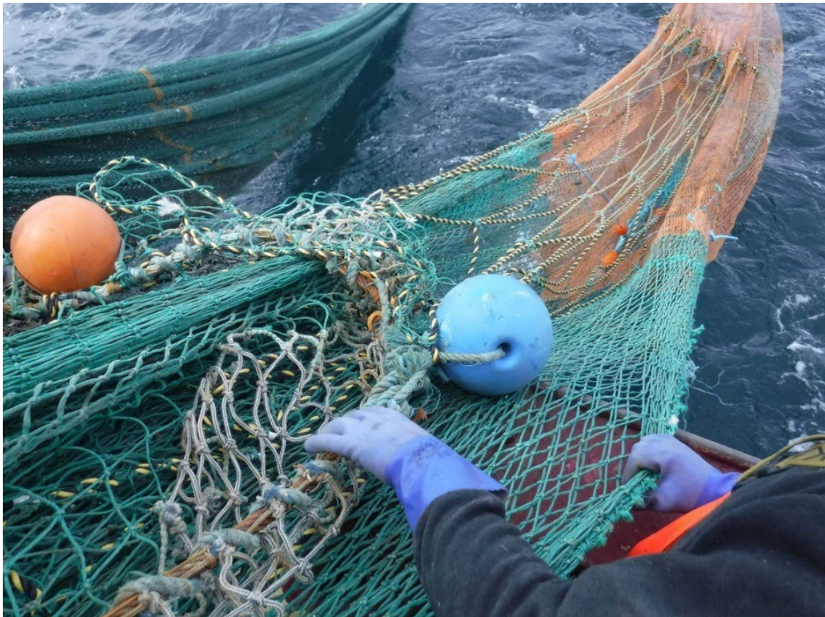
Figure 9. Photo showing an experimental net being trialled as part of the Northern Ireland Gear Trials project. The cover of this trawl has been cut out and replaced with a pelagic sized mesh (© Northern Ireland Gear Trial Project 2017-2022).
