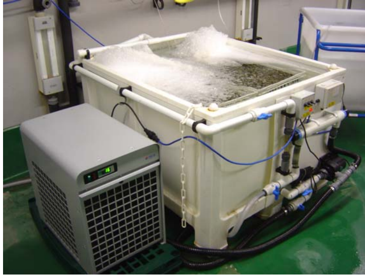
Figure 2: Experimental Depuration unit in operation, 90 kg of cockles at 16°C at 41h into cycle.
