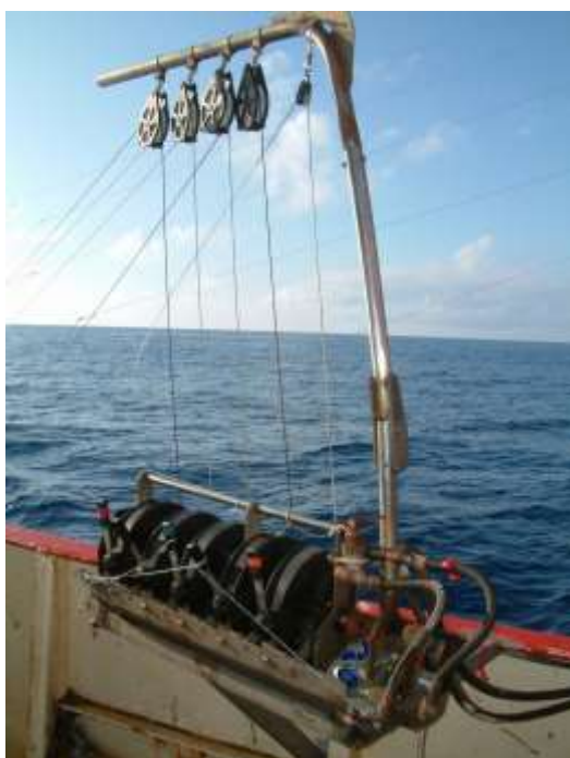
Figure 5 American style Tuna Tugs™ mounted on the port rail
