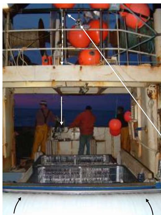
Figure 8 Shooting the longline; the line drum is at the bottom of the picture
