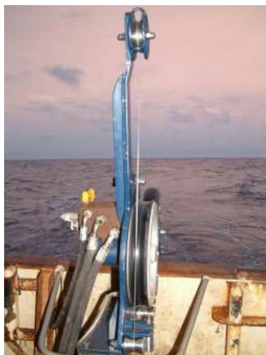
Figure 6 Longline equipment: Line setter mounted on the stern
