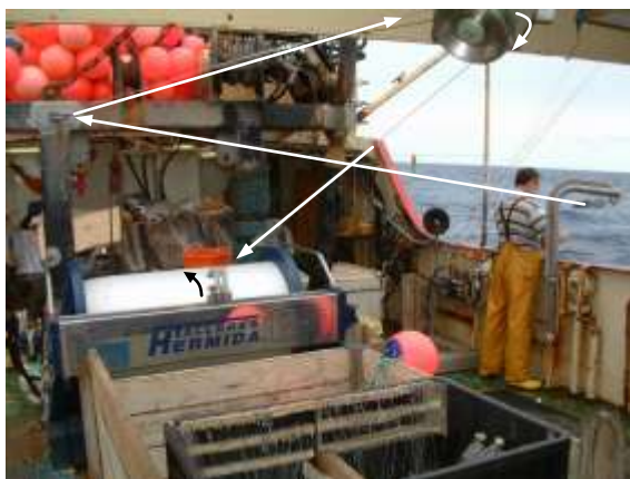
Figure 9 Hauling the longline, showing the path of the nylon monofilament
