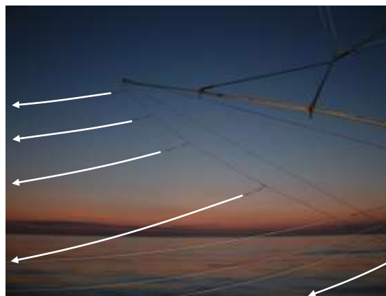
Figure 10 Pole on port side, showing 5 lines being streamed from rubber shock-cords
