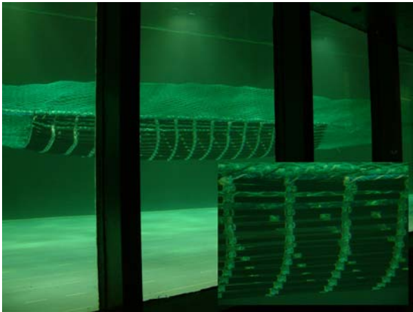
Figure 1: Flexi-panel™ with 25mm bar spacings (Variant 1)
