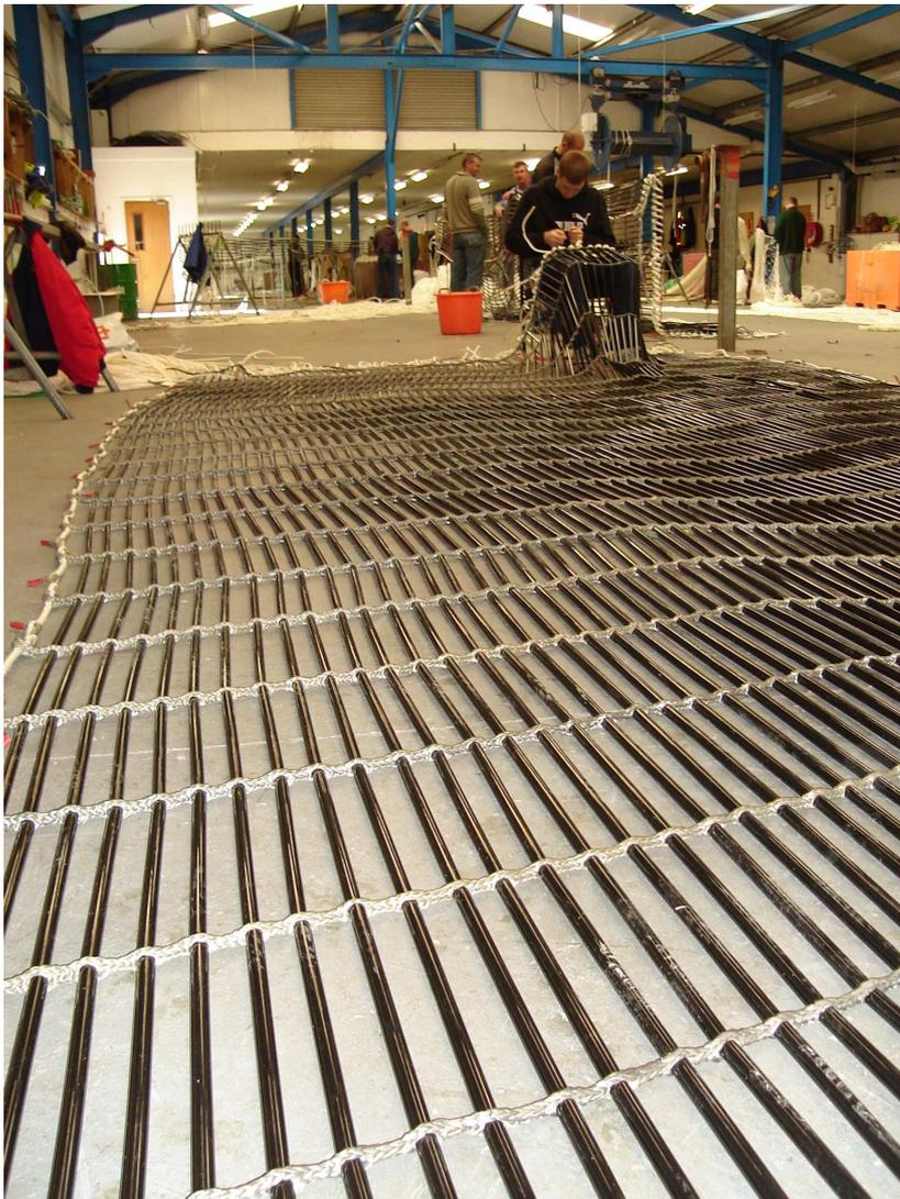
**Fig. 3 Grid construction showing nylon vertical bars and horizontal polysteel ropes (Photo: Swan Net-Gundry Ltd).**
