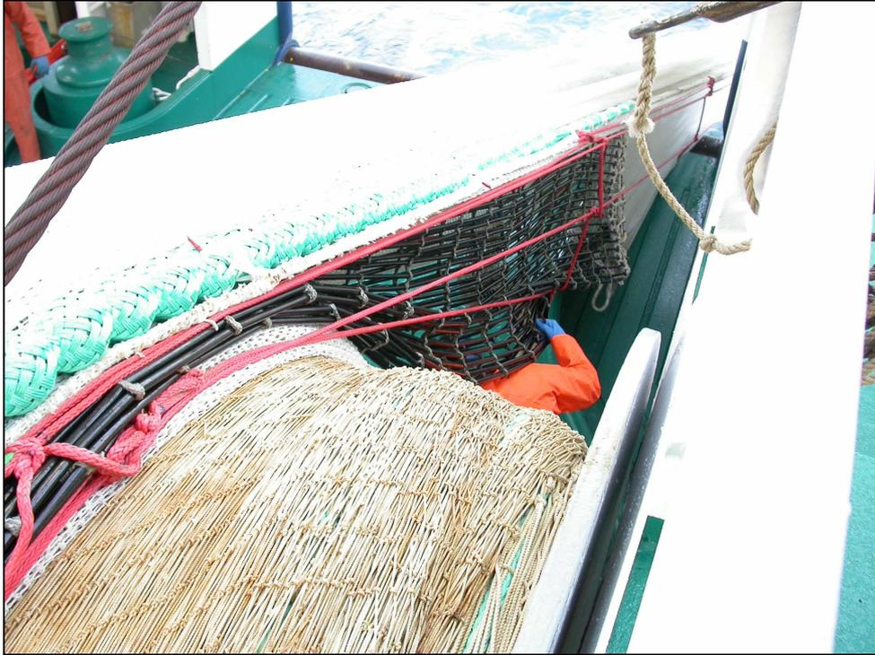
**Fig. 4 Grid section over the net-drum during shooting, illustrating flexibility. Open meshes constructed with 12 mm Nylex twine (red).**
